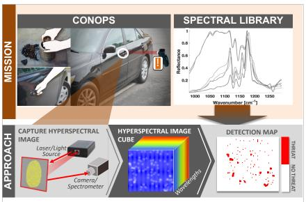
Figure 1. A notional depiction of standoff trace chemical classification concept of operations (CONOPS) via an active spectroscopic instrument. The reference signature library is pertinent to the system's ability to identify chemicals of interest.<sup>7</sup>
