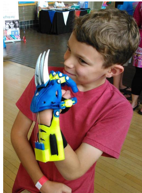
Figure 1: A 3D-printed upper-limb assistive technology device with extensive aesthetic modifications.
