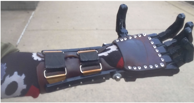
Figure 3: A customized, 3D-printed upper-limb assistive technology device in use (e-NABLE Talon hand design).
