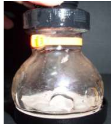
Figure 5.13 - Compliant boiling flask model used for validation (model is sitting on flat surface).
