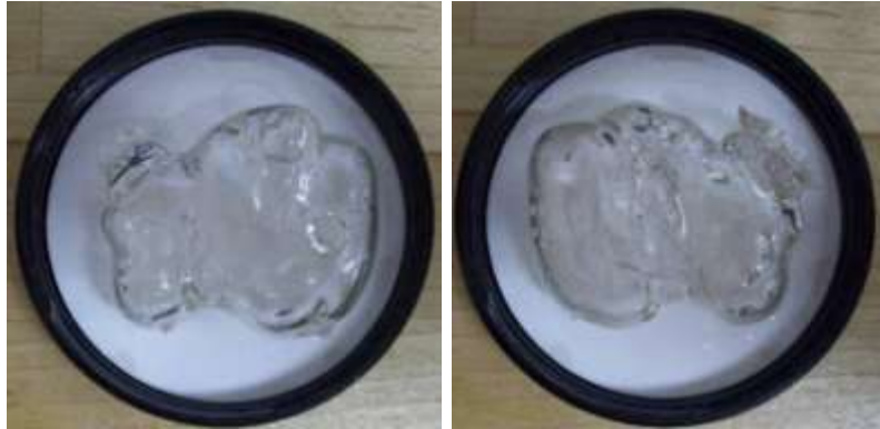
Figure 2.20 - Compliant experimental model of the emphysemic human lung.
