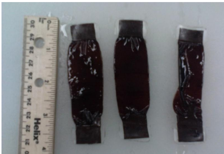
Figure 37: Hydrolyzed PAN samples with PDMS Grip Sections
