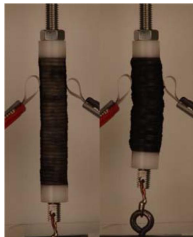
Figure 5: DEAP Stack Actuator in passive mode (left) and active mode (right) [16]
