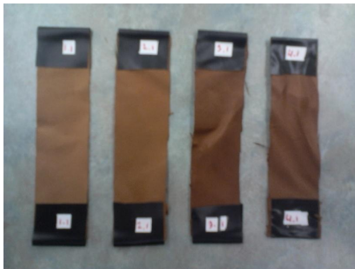
Figure 36: Annealed PAN nanofibers with increasing duration from left to right prepared for tensile testing
