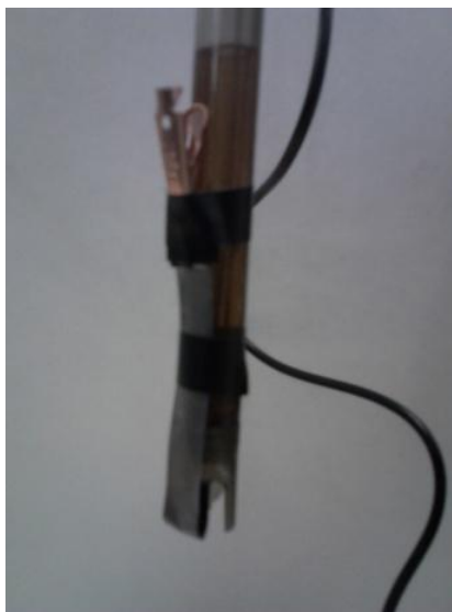
Figure 34: pH Meter with attached Graphite Sheet Electrode
