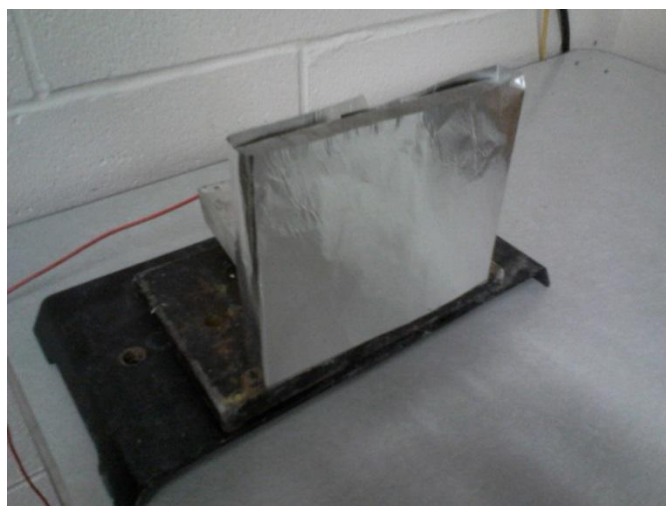
Figure 24: Close-up of Custom Collector Plate with Aluminum Foil
