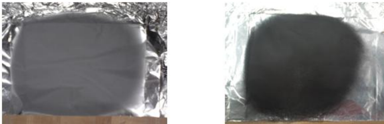
Figure 29: Top view of 90% PAN/10% MWCNT (left) and 66% PAN/33% Graphite (right) collected onto aluminum foil
