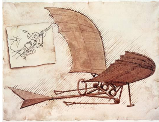
Figure 1: Leonardo da Vinci's plans for an Ornithopter, a flying machine kept aloft by the beating of its wings; about 1490 [2]
