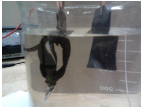
Figure 45: Graphite electrode buckling within PAN/Graphite/PAN composite
