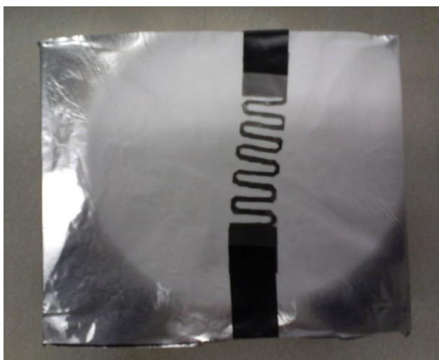
Figure 46: Modified Electrode Design applied to Electrospun Sample
