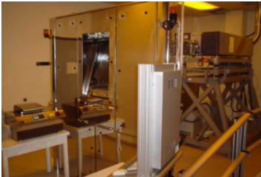
Figure 5. Exitech 193nm immersion projection system.
