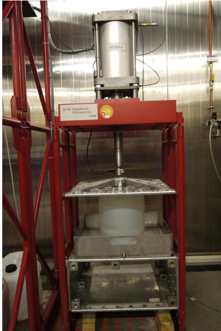
Figure 4: Stactic Stacking Machine
