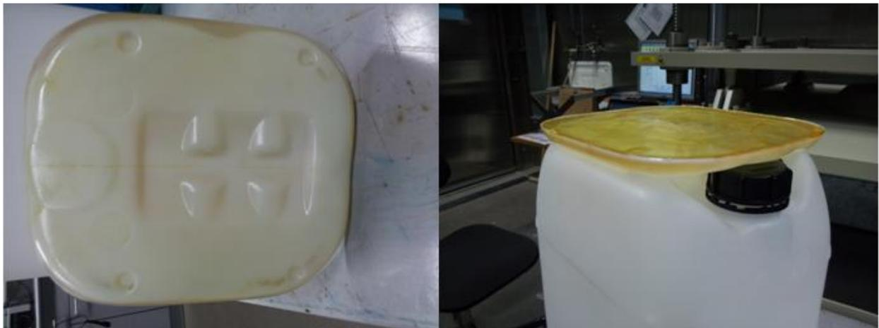
**Figure 2: Stacking Fixture**
