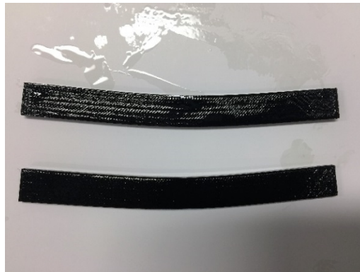
Figure 9: Two printed specimens after the deflection in the HDT testing
