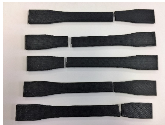
Figure 7: Clean-break of the fractured PLA specimens in tension
