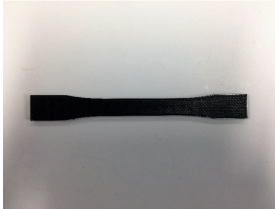
Figure 5: Tensile specimen of Type I printed by material extrusion (FDM)
