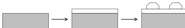
Figure 1.4: Self-assembly in the Stranski-Krastanov growth mode, through which epitaxial quantum dot growth is realized.
