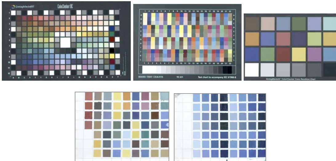
Figure 17. Color targets used in imaging experiment. Top row from left to right: ColorChecker DC, Esser, and ColorChecker. Bottom row: Gamblin and Blues. See Table III for a description of each target.
