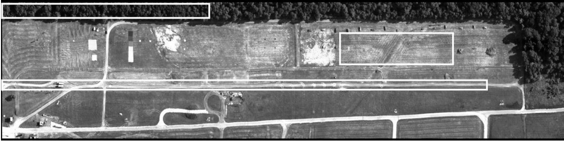
Figure 5. Grass, Tree, and Road sections from Run 5 for background covariance calculation
