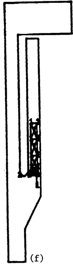
Figure 15 Propagation of Plastic Deformation Zone in Cantilever Pin at Various Loadings.
