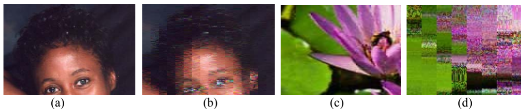
Figure 5. DYN files decompressed under the k_1 ordering (a) & (c) and decompressed under an alternate ordering (b) & (d), showing image degradation.
