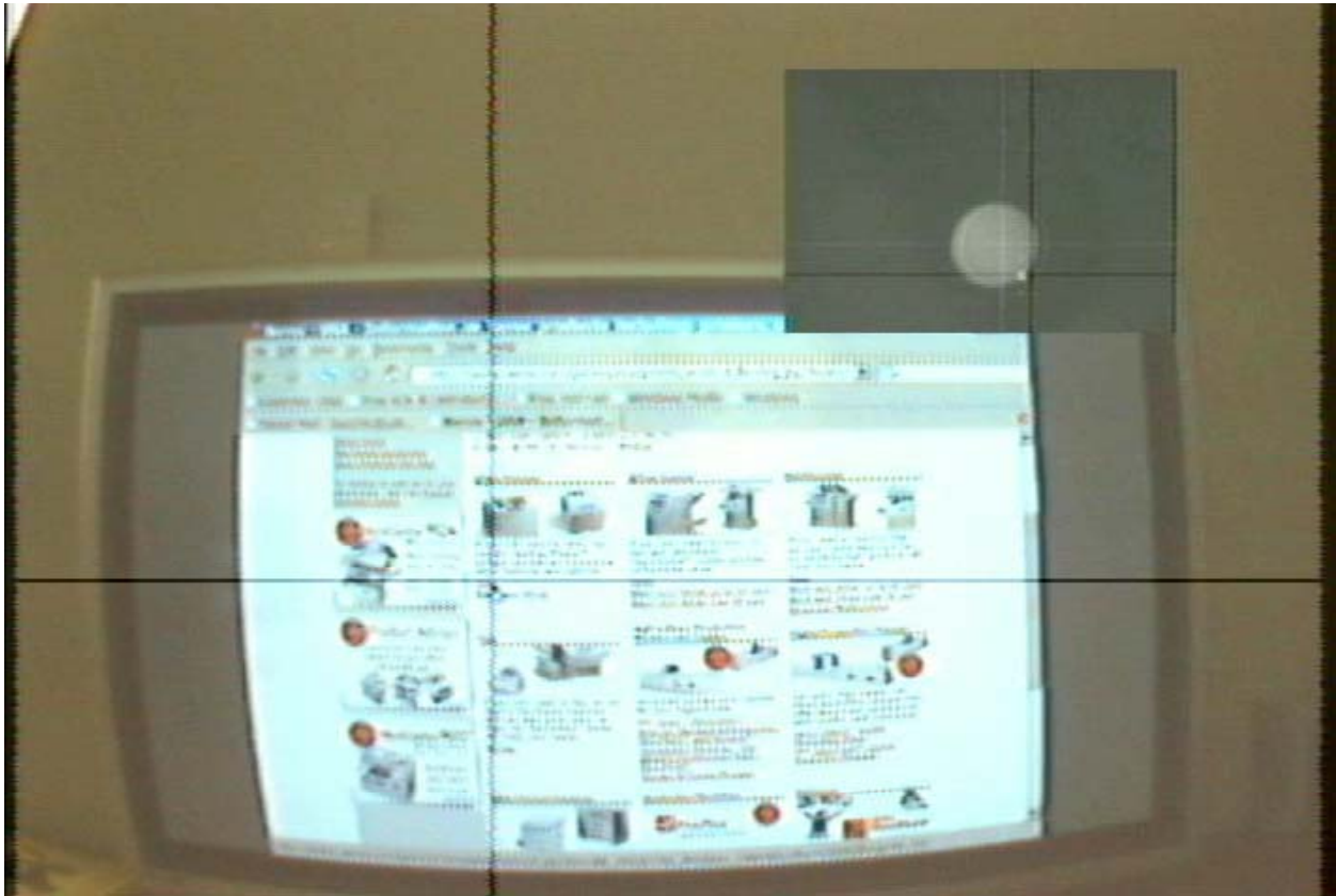
Figure 4: Scene Camera with Crosshairs Overlaid on the Screen and a picture-in-picture inset of the Eye Camera.
