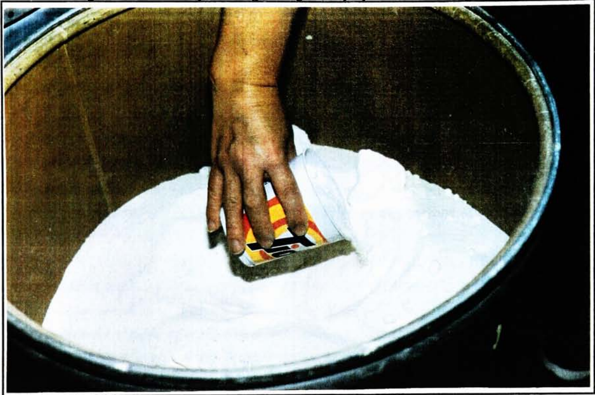
Figure 9: Durability Testing - Virgin Polystyrene Measuring Scoop
