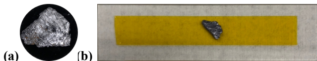
Figure 7: (a) MoS 2 chunk from SPI Supply (b) Bulk MoS 2 flake on double sided kapton tape waiting to be exfoliated
