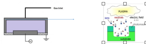
Figure 4. How Plasma is created for Dry Etching
