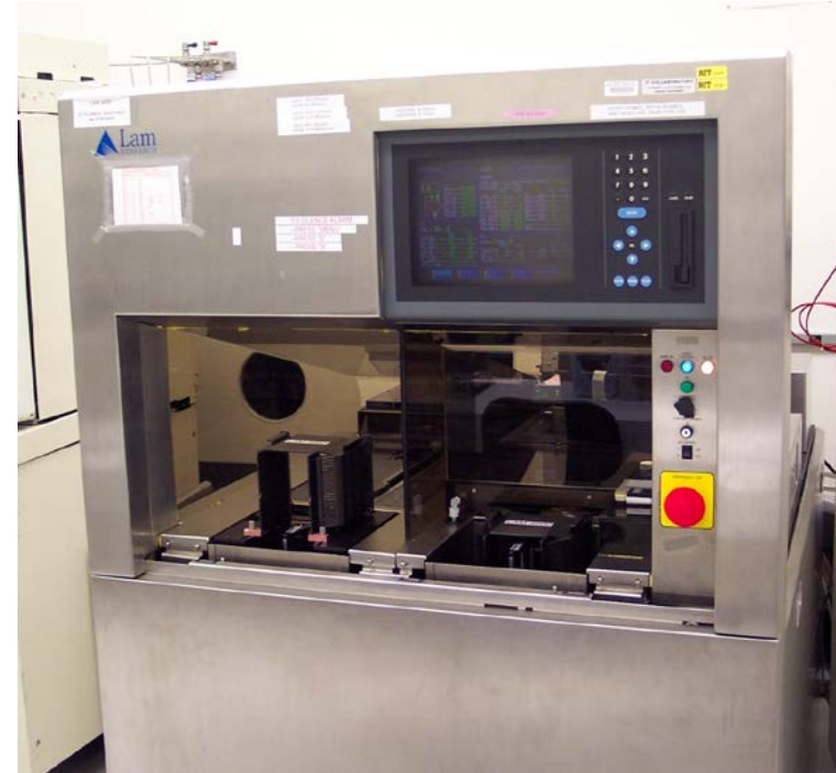
LAM 4600: Cl 2 RIE Etcher used for etching GaN
