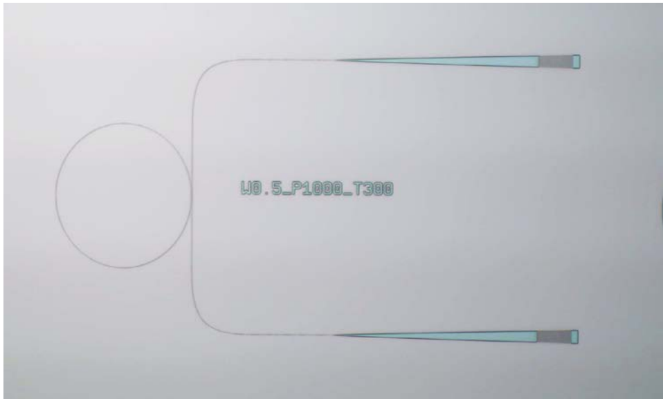
Fabricated Resonator Waveguide with 0.5\mu\text{m} width, 1\mu\text{m} coupler pitch, and 300\mu\text{m} coupler taper
