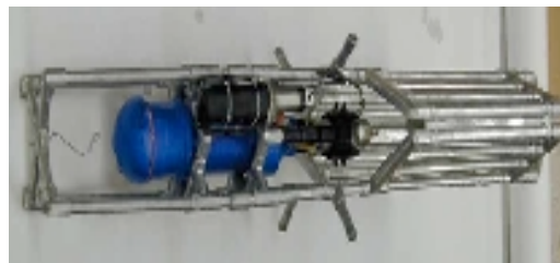
Figure 5. AQUATO, a Submersible Autonomous Robot for Underwater Data Gathering Proceedings of the 2003 American Society for Engineering Education Annual Conference & Exposition Copyright © 2003, American Society for Engineering Education
