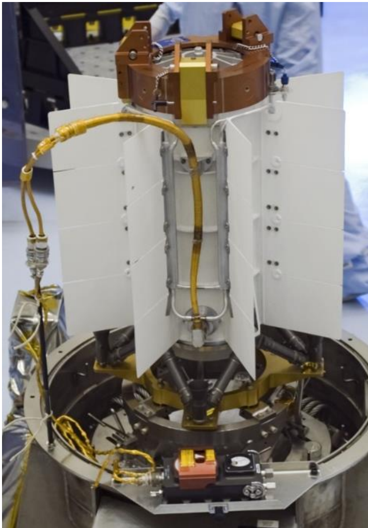
Figure 2 Multi-Mission Radioisotope Thermal Generator used by NASA capable of generating 110 Watts of electrical power.
