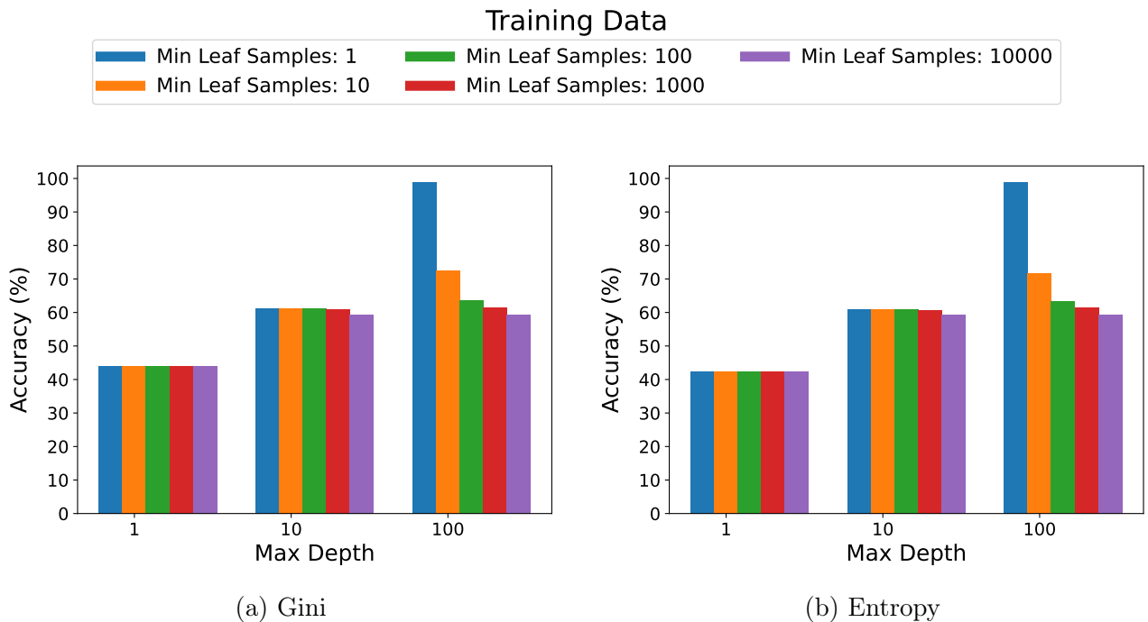
Figure 15: Bar graph of hyperparameter optimization for Decision Tree testing on the training data. a) shows with criterion=gini and b) shows criterion=entropy. The features used are White's Rating, Black's Rating, White's Win Rate, Black's Win Rate, White's Draw Rate, and Black's Draw Rate. The best accuracy is 98.79% which came from the hyperparameters {criterion=gini, max depth=100, minimum leaf samples=1}.
