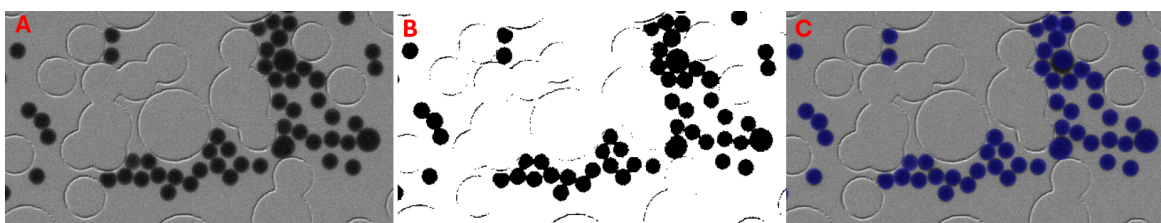
Figure 6.1: Circle Hough Transform Detection Method A) Background Subtraction and stabilization B) Adaptive Binarization C) Circle Hough Transform Detection
