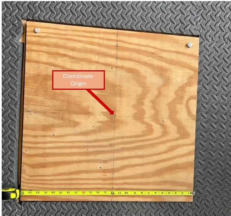
Figure 9: Image of force plate wooden board with tape measure showing length of 24 inches (609.6mm). The arrow points to the origin of the coordinate system aligning with stabilogram centers.
