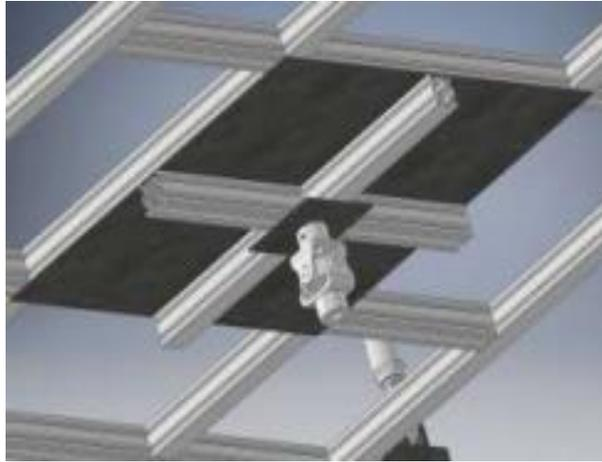
Figure 4: U-joint under center of BASE platform.
