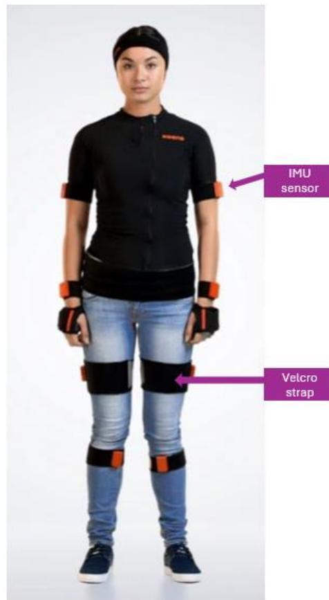
Figure 15: The Xsens MVN Awinda IMU system (Movella, Henderson NV) consisting of 17 wireless IMU sensors attached via velcro strips.
