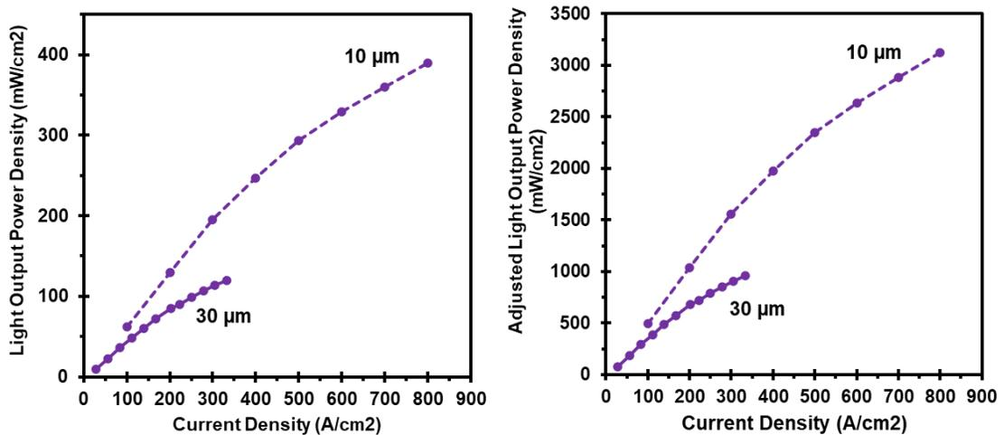
Figure 4.4.10: Measured (a) and adjusted (b) light output power as a function of current density for 10  $\mu\text{m}$  (dashed) and 30  $\mu\text{m}$  (solid)  $\mu\text{LEDs}$ .
