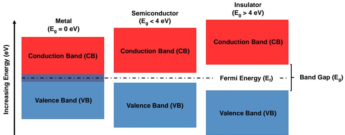
Figure 1.1.1: Conduction (CB) and valence (VB) band alignments for metals, semiconductors, and insulators.
