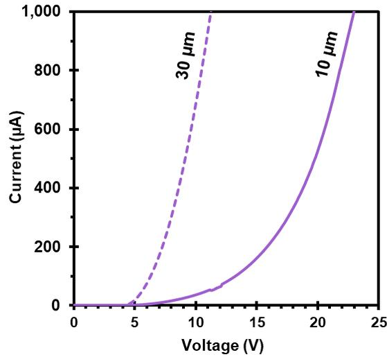
Figure 4.4.9: Current voltage characteristics for 30  $\mu\text{m}$  and 10  $\mu\text{m}$   $\mu\text{LEDs}$  between 0 and 25 V.
