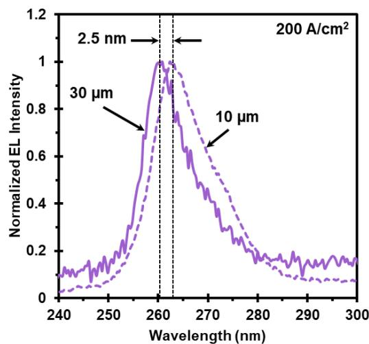
Figure 4.4.8: Normalized EL spectra for individual 30  $\mu\text{m}$  and 10  $\mu\text{m}$   $\mu\text{LEDs}$  at 200  $\text{A}/\text{cm}^2$ .
