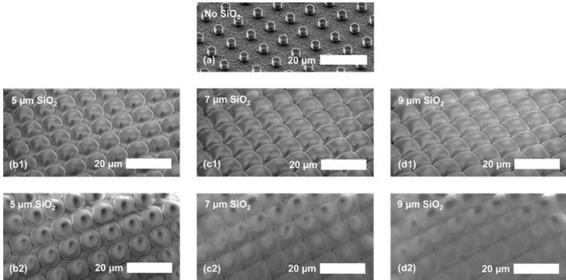
Figure 3.7.1: SEM images showing micropillars (2.5  $\mu\text{m}$  diameter, 2  $\mu\text{m}$  height, 10  $\mu\text{m}$  pitch) following dry etching and KOH treatment (a), and subsequently after 5  $\mu\text{m}$  (b), 7  $\mu\text{m}$  (c), and 9  $\mu\text{m}$  (d) of conformal TEOS deposition. Images a, b1, c1, and d1 were taken at 45° off normal, while b2, c2, and d2 were taken normal to the sample surface [18].
