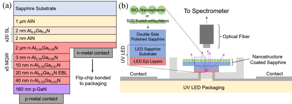
Figure 5.5.6: (a) Cross-sectional view of the UV LED epitaxial structure used to test  $\eta_{\text{EXT}}$  through nanosphere and nanohemisphere arrays. (b) Cross-sectional view of the angle-dependent EL setup used to measure normalized  $\eta_{\text{EXT}}$  through a nanostructure-on-sapphire sample.
