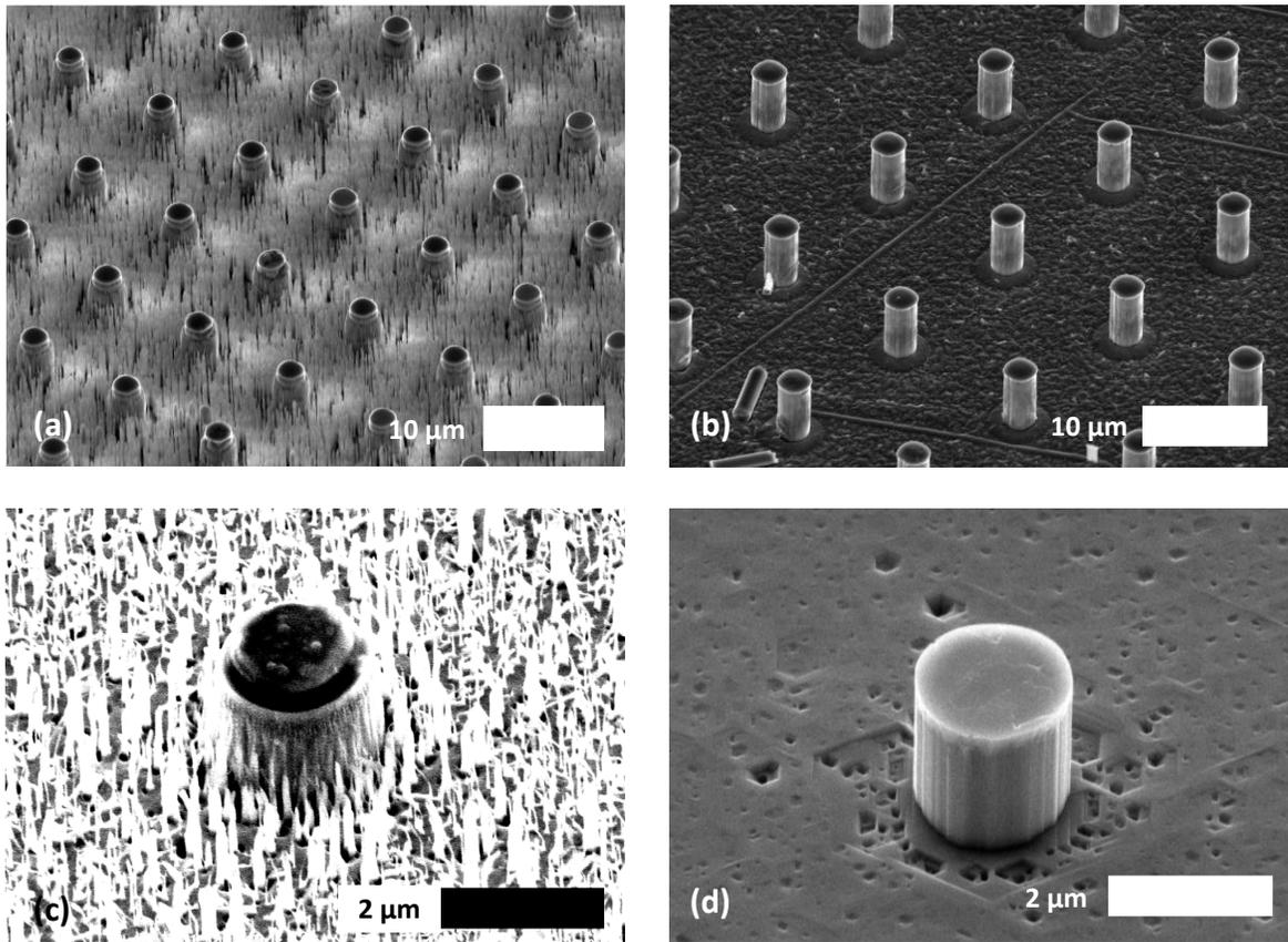
Figure 3.5.1: GaN nanowires before (a, c) and after (b, d) a 30 min etch in 2 wt.% KOH at 80°C.
