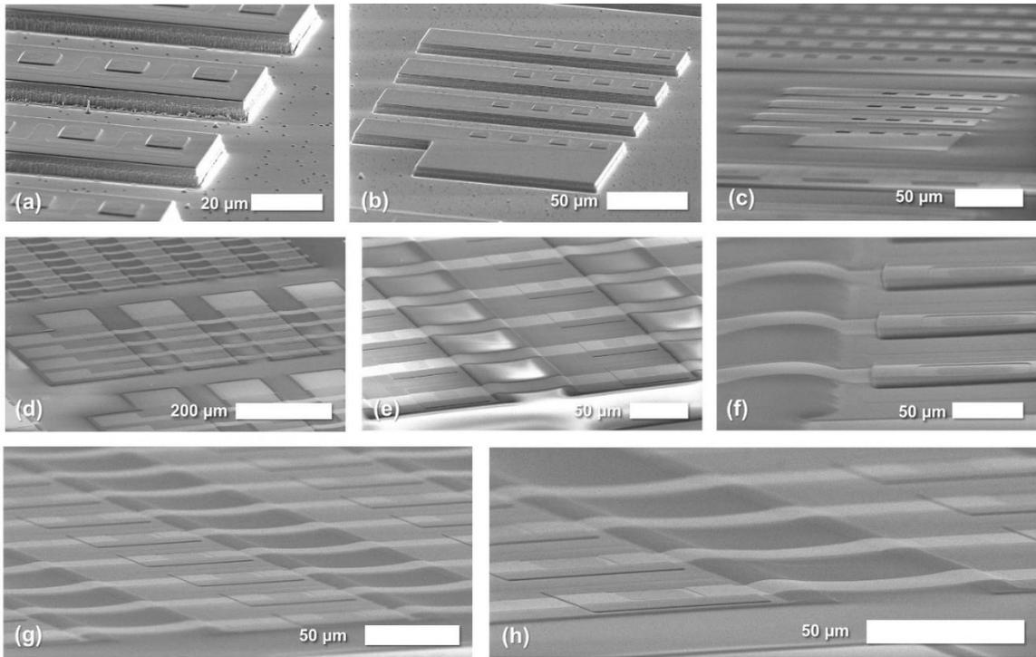
Figure 5.3.4: SEM images showing passive matrix displays prior to trench planarization (a,b), following trench planarization (c), and following p-interconnect formation (d-h). (a, b, d, and e) are imaged at 70° off-normal, while (c, f, g, and h) are imaged at 80° off-normal.
