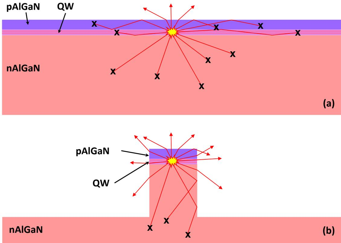
Figure 2.2.1: Schematic showing extraction (arrow) or absorption (x) of light in a planar mesa DUV LED (a), and a nanowire DUV LED (b).
