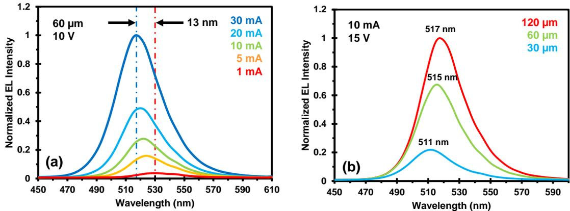
Figure 5.3.7: (a) Blueshift characteristics for a 60  $\mu\text{m}$   $\mu\text{LED}$  driven at 10 V and 1-30 mA. A blueshift of 13 nm is observed when drive current is increased from 1 mA to 30 mA. (b) Size dependent EL characteristics for devices driven at 10V and 10 mA. A moderate blueshift of 6 nm is observed between the 30  $\mu\text{m}$  and 120  $\mu\text{m}$   $\mu\text{LED}$ s.
