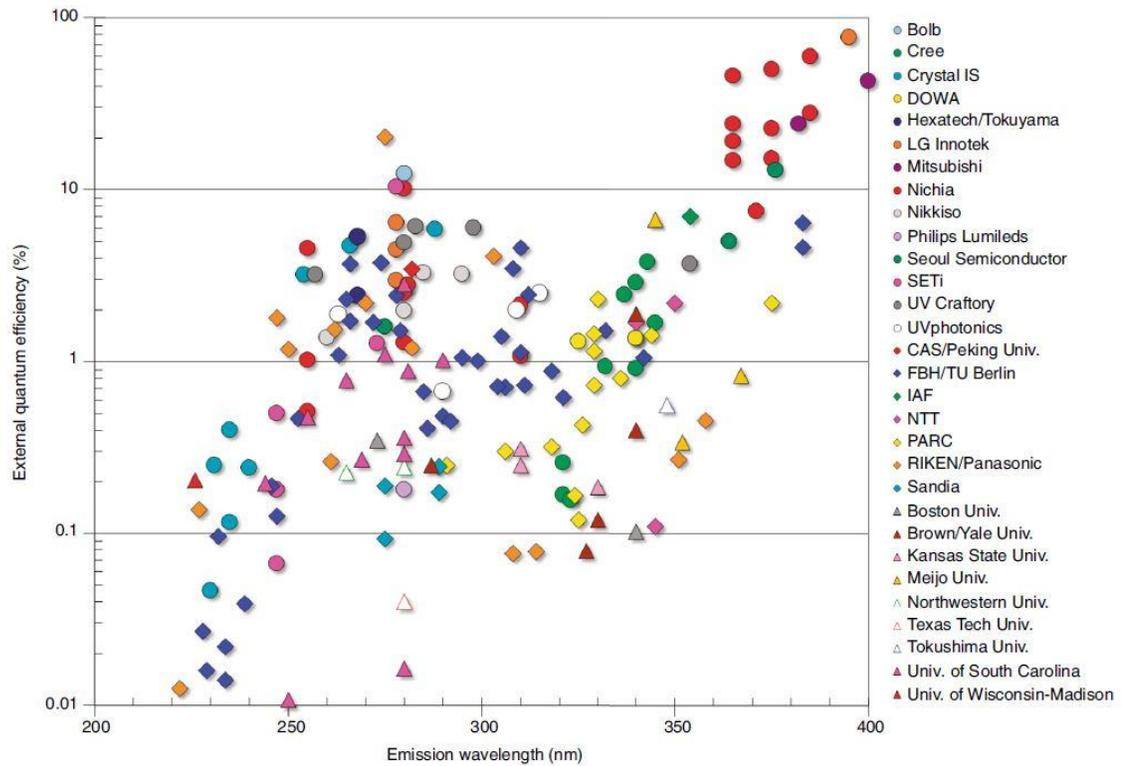
Figure 2.1.1: EQEs of planar UV LEDs developed in the past 20 years, showing the trend of EQE increasing with wavelength. The dip in EQE around 320 nm is due primarily to lack of research interest in this wavelength range. Reprinted with permission [1].
