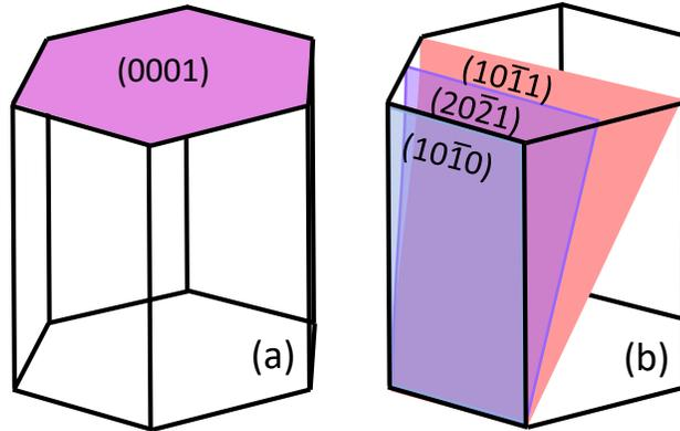
Figure 4.2.3: (a) Wurtzite unit cell highlighting the (0001) c-plane surface, (b) wurtzite unit cell highlighting the  $(10\bar{1}0)$  m-plane and semi-polar planes attacked by the AZ400K etch.
