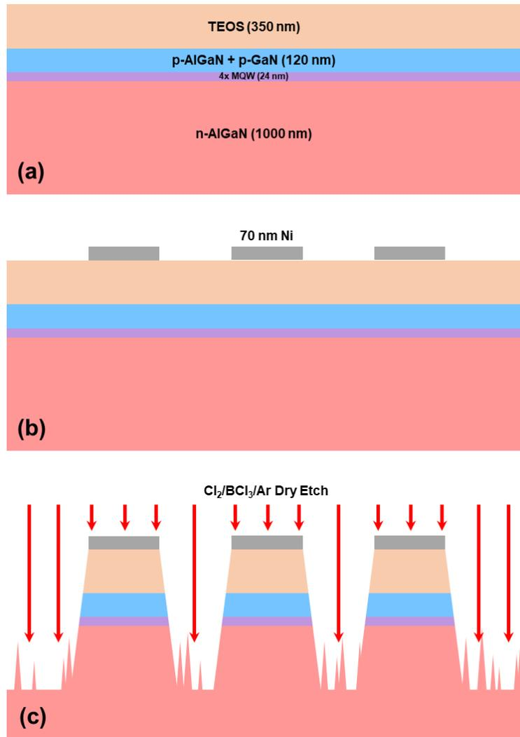
Figure 4.5.6(a-c): Deposition of 350 nm TEOS (a), patterning of 70 nm Ni (b), dry etching of the TEOS and underlying AlGaIn epitaxy (c).
