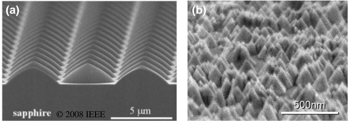
Figure 2.1.2: SEM images showing a patterned sapphire substrate (a) [17] and surface roughening of GaN (b) [13]. Reprinted with permission [13, 17].
