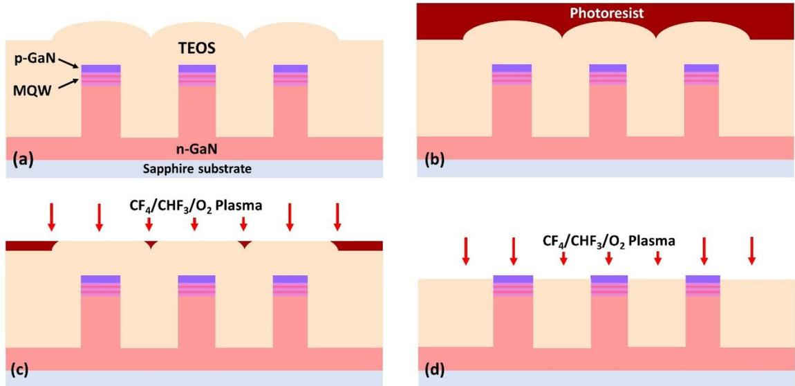
Figure 3.7.2: Cross-sectional diagram of the dielectric planarization process. (a) TEOS deposited conformally over GaN nanowires via PECVD. (b) Coating of a self-planarizing photoresist layer over the TEOS surface. (c) Etch back of the photoresist and TEOS using a CF<sub>4</sub>/CHF<sub>3</sub>/O<sub>2</sub> plasma which etches both materials at ~70 nm/min. (d) Planarized SiO<sub>2</sub> etched back to expose the p-GaN tips of the nanowires [18].
