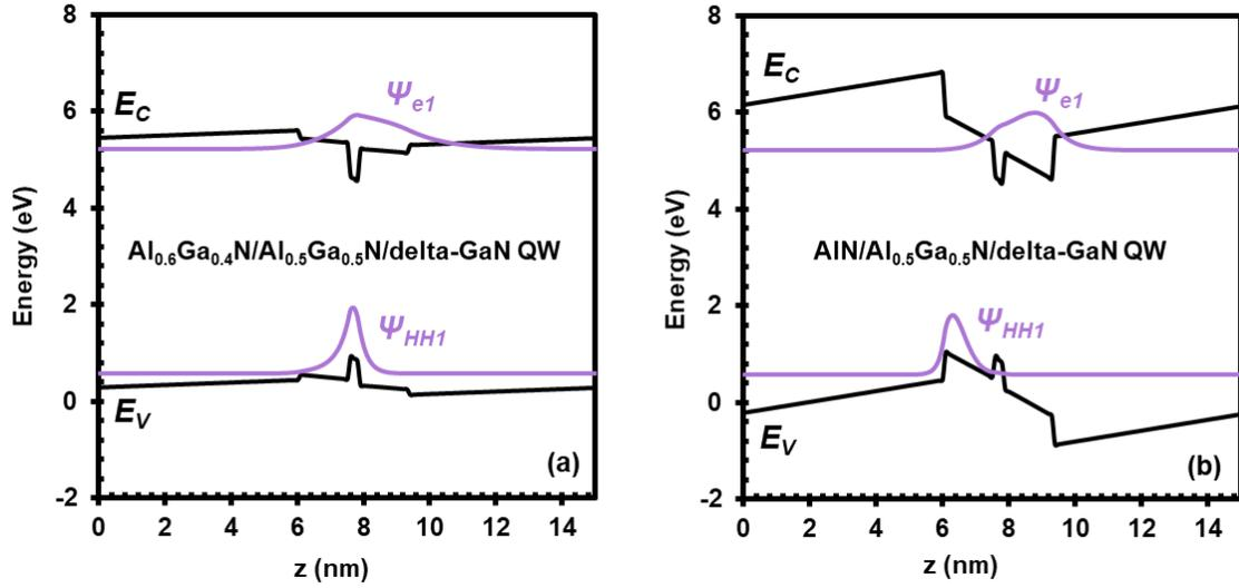
Figure 4.4.1: Bandstructures with overlaid electron and hole wavefunctions of a  $\text{Al}_{0.6}\text{Ga}_{0.4}\text{N}/\text{Al}_{0.5}\text{Ga}_{0.5}\text{N}/\text{delta-GaN}$  QW (a) and a  $\text{AlN}/\text{Al}_{0.5}\text{Ga}_{0.5}\text{N}/\text{delta-GaN}$  QW (b).
