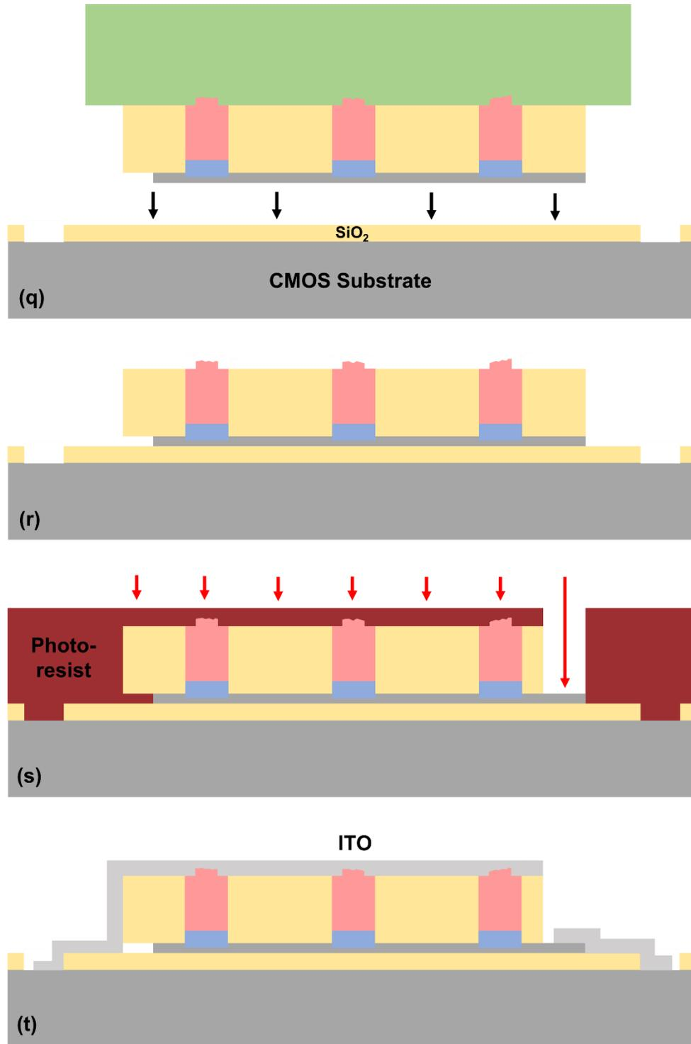
Figure 4.6.1(q-t): Lower of the inverted device onto the CMOS host substrate (q, r), etching of contact opens through the planarized  $\text{SiO}_2$  to allow access to the Ni p-contact (s), and deposition of an interconnect layer (either Ni or ITO) to connect the device with the CMOS host substrate (t).
