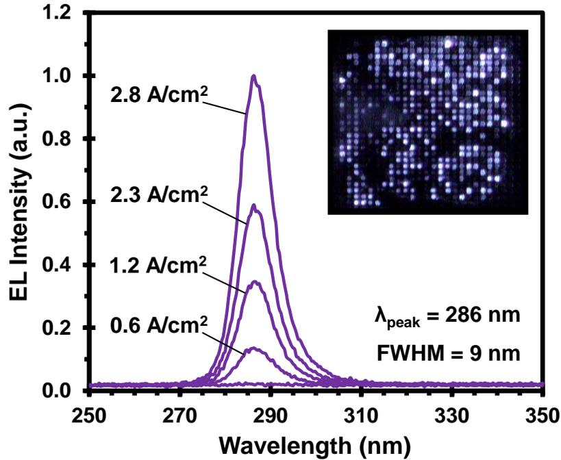
Figure 4.1.5: EL spectra of a 30x30 nanowire array LED at various current densities.  $\lambda_{\text{peak}}$  is located at 286 nm and all spectra have a linewidth of 9 nm. The inset shows an optical image of the illuminated nanowire array.
