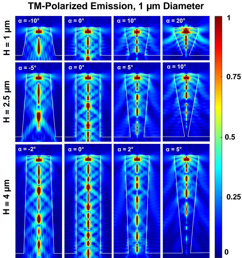
Figure 4.3.5: Cross-sectional electric field intensity plots for 1  $\mu\text{m}$ , 2.5  $\mu\text{m}$ , and 4  $\mu\text{m}$  tall structures with diameters of 1  $\mu\text{m}$  and taper angles between  $-10^\circ$  and  $20^\circ$  for TM-polarized emission at  $\lambda = 270 \text{ nm}$ .
