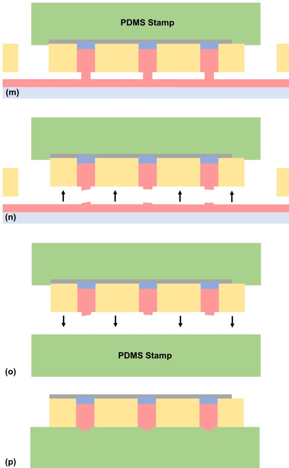
Figure 4.6.1(m-p): Contacting of the PDMS stamp to a device (m), lifting of the device from the substrate (n), lowering (o) and placing (p) of the device onto a second PDMS stamp.
