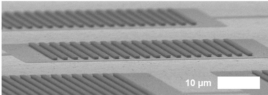
Figure 4.5.8: SEM images of a 20x20 array of 1.25  $\mu\text{m}$  micropillars on a 2.5  $\mu\text{m}$  pitch following n-metal deposition.
