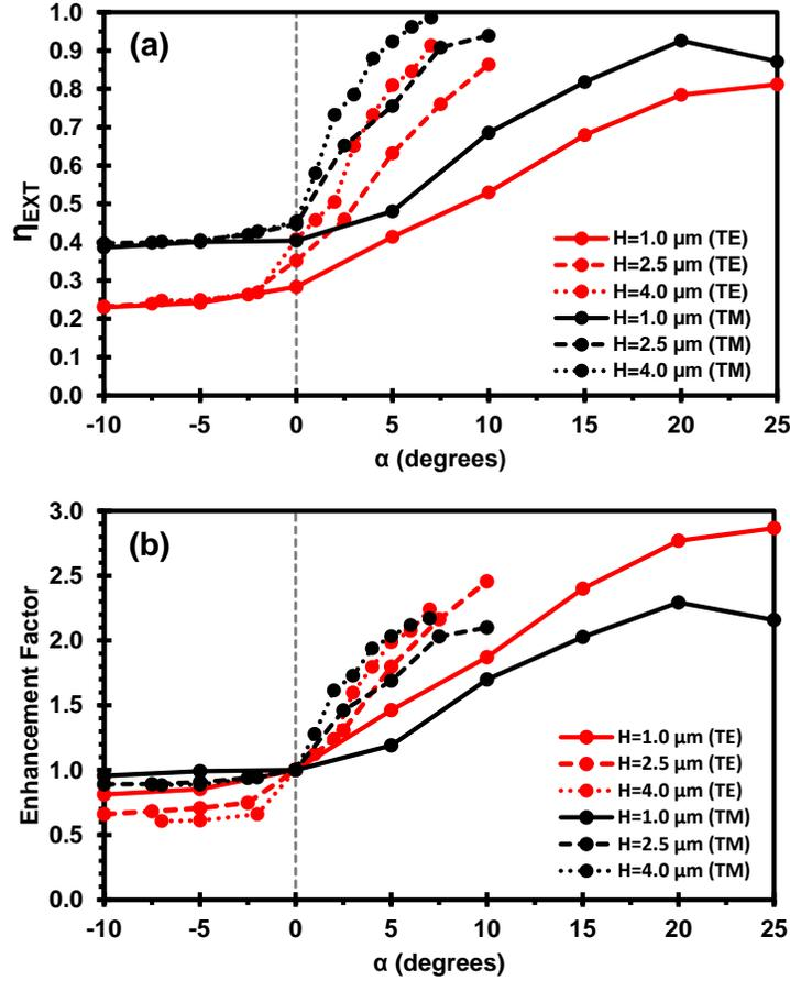
Figure 4.3.3:  $\eta_{\text{EXT}}$  (a) and  $\eta_{\text{EXT}}$  enhancement factor (b) for TE (red) and TM (black) polarizations as a function of taper angle  $\alpha$  for 1  $\mu\text{m}$  tall (solid), 2.5  $\mu\text{m}$  tall (dashed), and 4  $\mu\text{m}$  tall (dotted) structures with diameters of 1  $\mu\text{m}$  at  $\lambda = 270 \text{ nm}$ .
