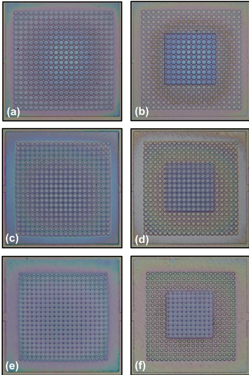
Figure 4.5.17: Optical images of completed devices of full and reduced size. (a) and (b) show 3  $\mu\text{m}$  micropillars on a 5  $\mu\text{m}$  pitch, (c) and (d) show 2  $\mu\text{m}$  micropillars on a 3  $\mu\text{m}$  pitch, and (e) and (f) show 1  $\mu\text{m}$  micropillars on a 2  $\mu\text{m}$  pitch.
