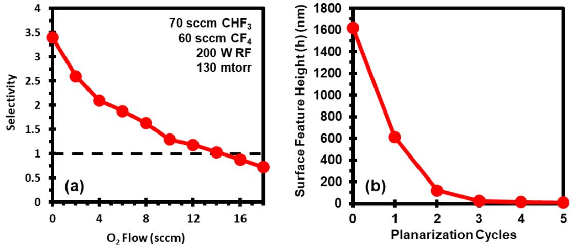
Figure 4.5.3: (a) Etch selectivity between photoresist and TEOS as a function of the O<sub>2</sub> flow rate in sccm. (b) Surface feature height *h* (see Figure 4.5.2(a)) as a function of the number of planarization cycles [104].
