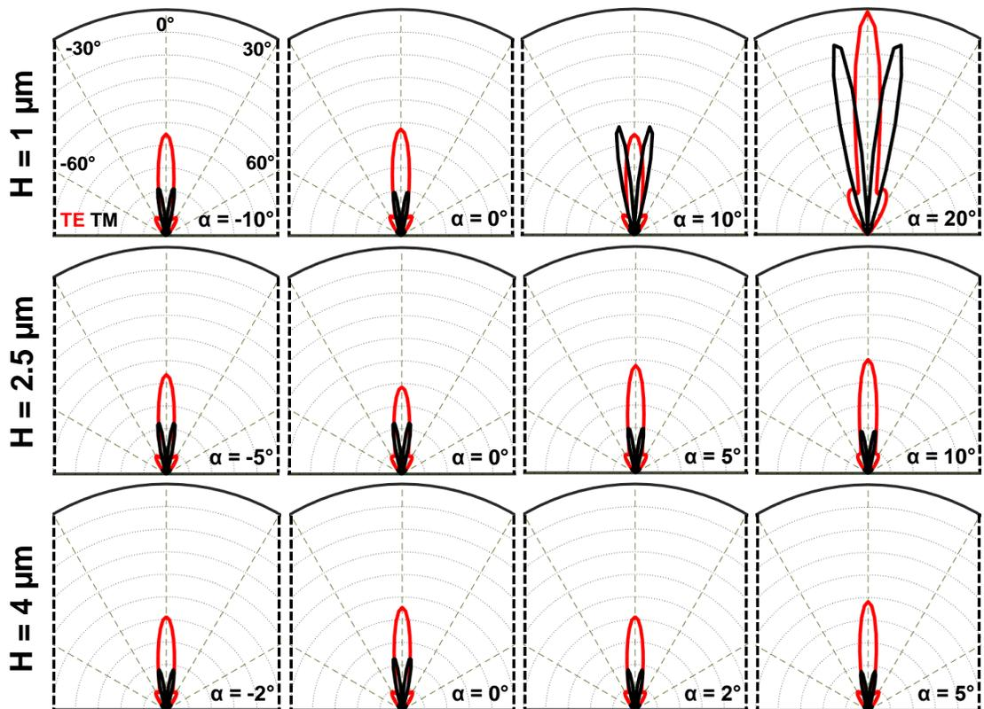
Figure 4.3.6: Far-field emission patterns for TE-polarized (red) and TM-polarized (black) light, for  $1\ \mu\text{m}$ ,  $2.5\ \mu\text{m}$ , and  $4\ \mu\text{m}$  tall structures with diameters of  $1\ \mu\text{m}$  and taper angles between  $10^\circ$  and  $20^\circ$  at  $\lambda = 270\ \text{nm}$  (the same structures whose electric field intensity plots are shown in Figures 4.3.4 and 4.3.5).
