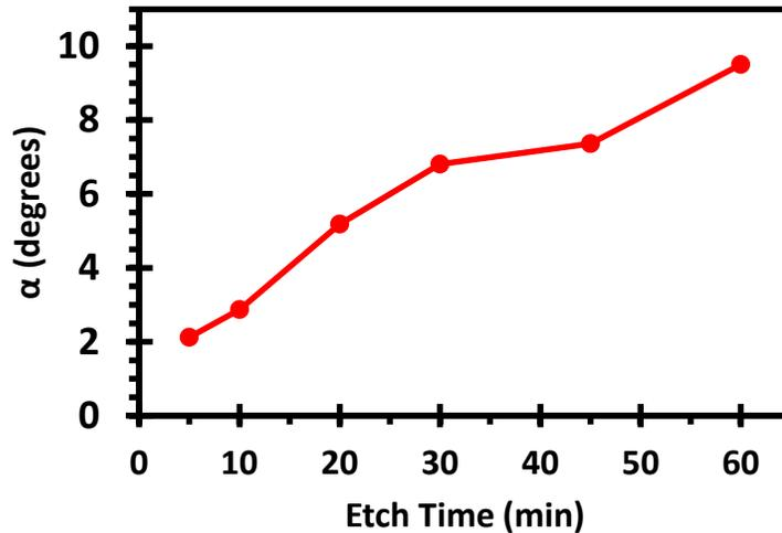
Figure 4.1.4: Nanowire taper angle as a function of etch time. Taper angles beyond  $10^\circ$  could not be measured due to the size of the nanowires.
