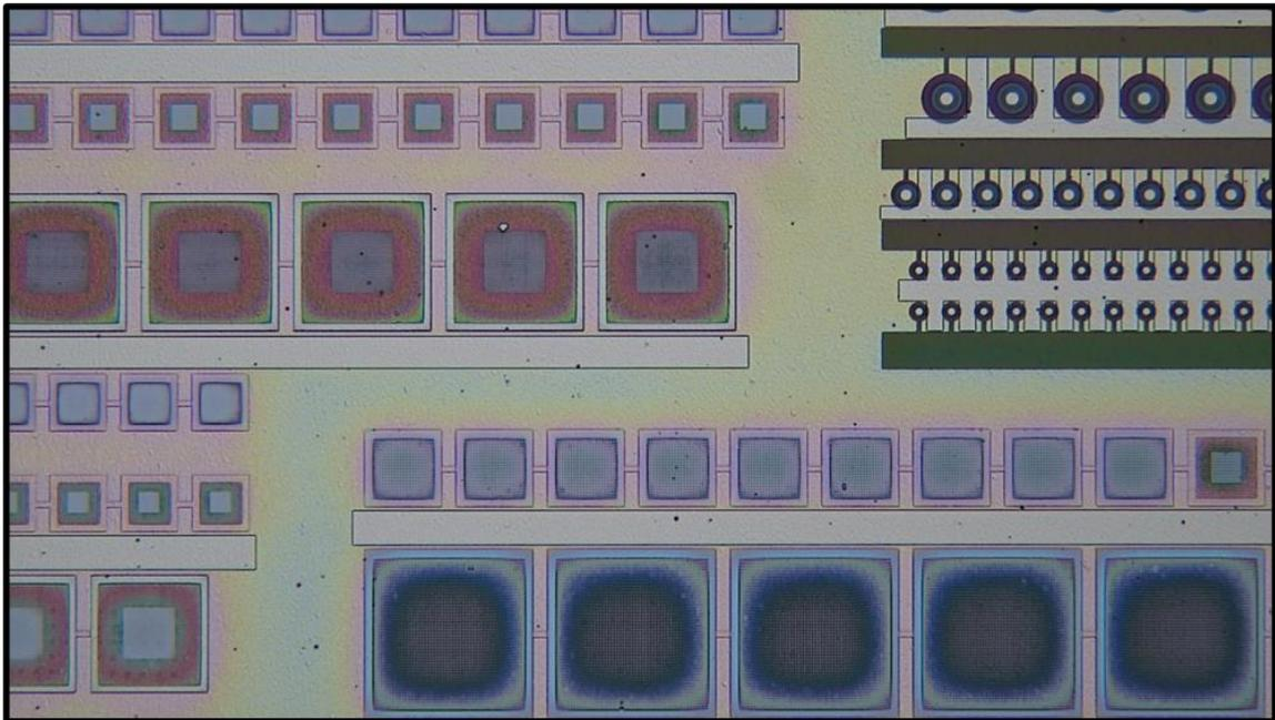
Figure 4.5.16: Optical images of completed devices. The variable color of different arrays is caused by thin film interference in the variable thickness TEOS interlayer of the arrays. Conventional mesa LEDs can be seen in the top right.
