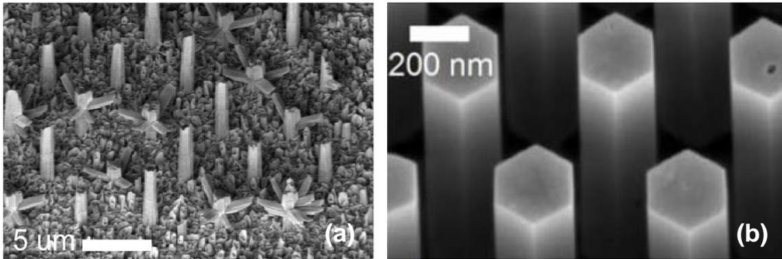
Figure 2.2.3: SEM images of epitaxial AlGaN nanowires grown using MBE and selective area epitaxy. Reprinted with permission [68, 69].
