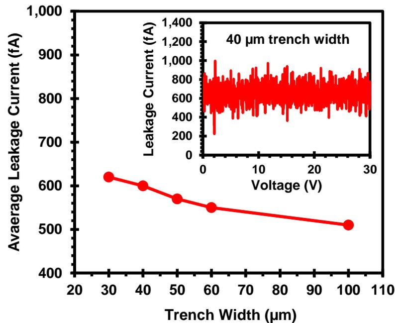
Figure 5.3.5: Leakage current as a function of trench width. (inset) Leakage current as a function of applied bias for a 40  $\mu\text{m}$  wide trench.
