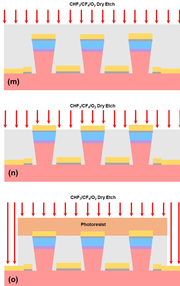
Figure 4.5.6(m-o): Etchback of the planarized TEOS surface (m), exposure of the micropillars (n), etching of the field TEOS to expose the n-contact (o).
