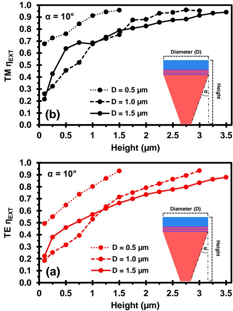
Figure 4.3.7:  $\eta_{EXT}$  for TM (a) and TE (b) polarizations as a function of height for structures with diameters of 0.5  $\mu\text{m}$ , 1  $\mu\text{m}$ , and 1.5  $\mu\text{m}$  and (solid), 2.5  $\mu\text{m}$  tall (dashed), and 4  $\mu\text{m}$  tall (dotted) structures with diameters of 1  $\mu\text{m}$  at  $\lambda = 270 \text{ nm}$ .
