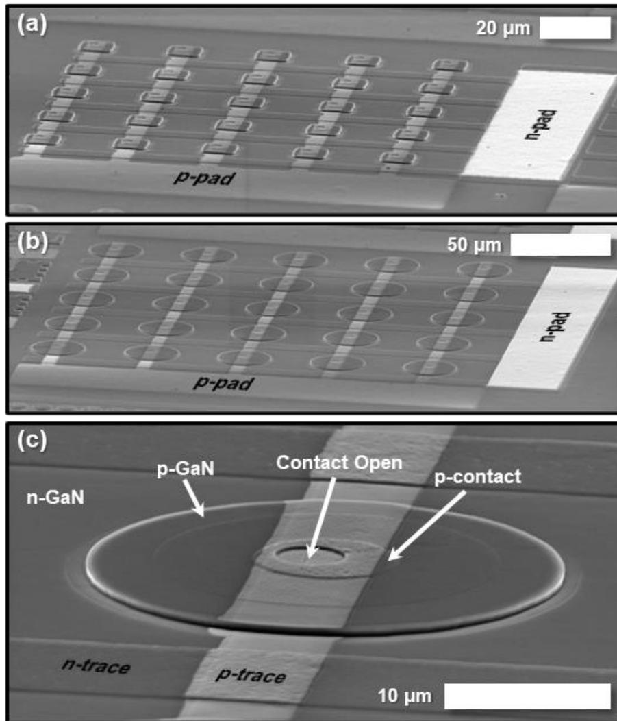
Figure 4.4.4: SEM images of completed 10  $\mu$ m (a) and 30  $\mu$ m (b, c)  $\mu$ LEDs. Images taken at 80° off normal. p- and n-pads are shown in (a, b) while p- and n-traces, nGaN/pGaN regions, and the locations of contact opens and p-contacts are shown in (c).
