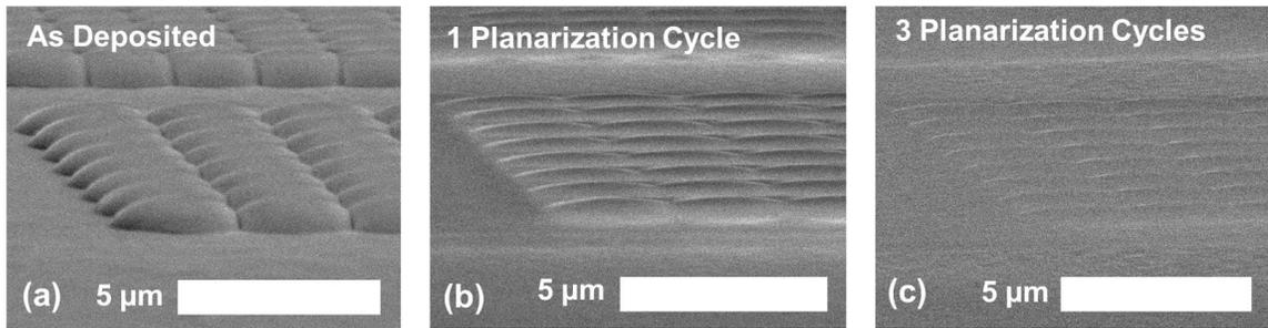
Figure 4.5.10: SEM images showing the TEOS surface over the same micropillar array as deposited (a), and after 1 (b) and 3 (c) planarization cycles.
