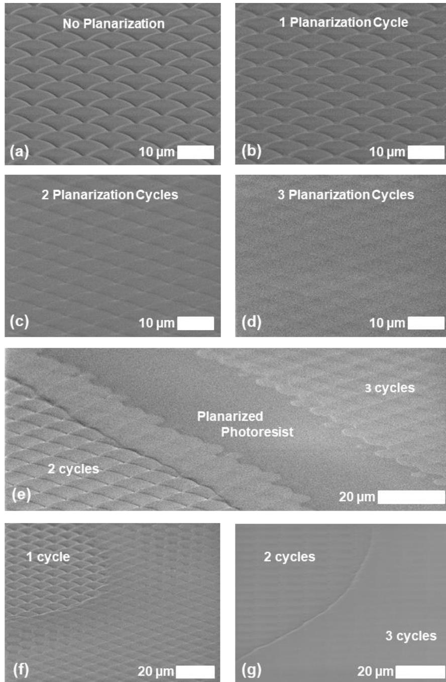
Figure 4.5.4: SEM images showing the TEOS surface after (a) no planarization, (b) 1 planarization cycle, (c) 2 planarization cycles, (d) and 3 planarization cycles. (e) Shows a region in which 2 and 3 cycles of planarization are visible, as well as residual photoresist between the two regions. Likewise (f) and (g) do the same for direct comparison of 1 and 2 cycles and 2 and 3 cycles respectively. All images were taken at 70° off normal [104].
