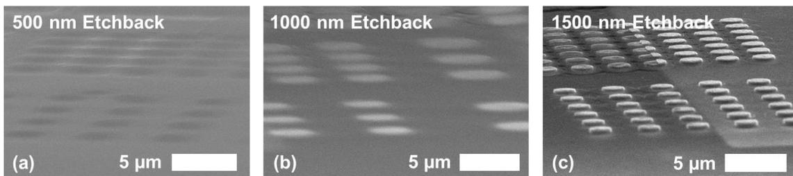
Figure 4.5.11: SEM images showing the TEOS surface over micropillar arrays following 500 nm etchback (a), 1000 nm etchback (b), and 1500 nm etchback (c).
