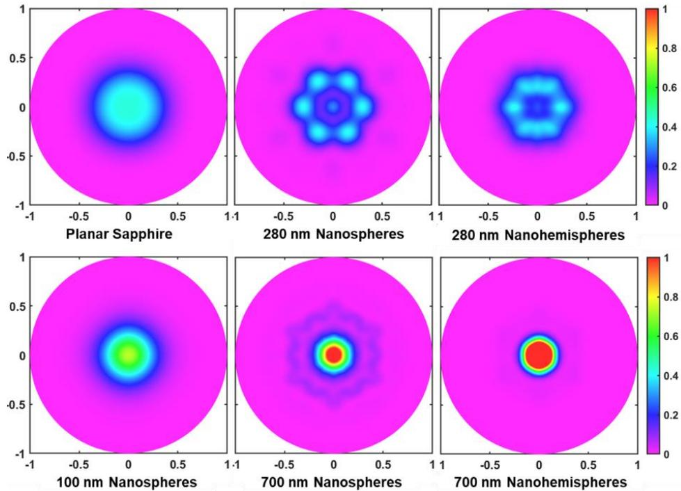
Figure 5.5.4: Far field radiation intensity patterns for simulation structures of variable nanosphere and nanohemisphere diameters showing spatial variation in far field radiation intensity with nanostructure diameter. The centers of these plots ( $x = y = 0$ ) represent emission at  $0^\circ$  off-normal while the plot edges ( $x = y = \pm 1$ ) represent emission at  $90^\circ$  off-normal.
