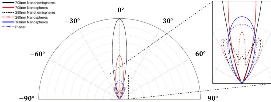
Figure 5.5.5: Overlaid polar intensity plots of the far field radiation intensity data presented in Figure 5.5.4, allowing for easier quantitative comparison of simulation structures with variable nanosphere and nanohemisphere diameters.
