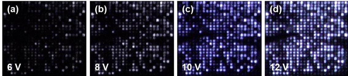
Figure 4.1.6: EL spectra of a 30x30 nanowire array LED at 6, 8, 10, and 12 V, showing the inconsistent manner in which individual nanowires illuminate.
