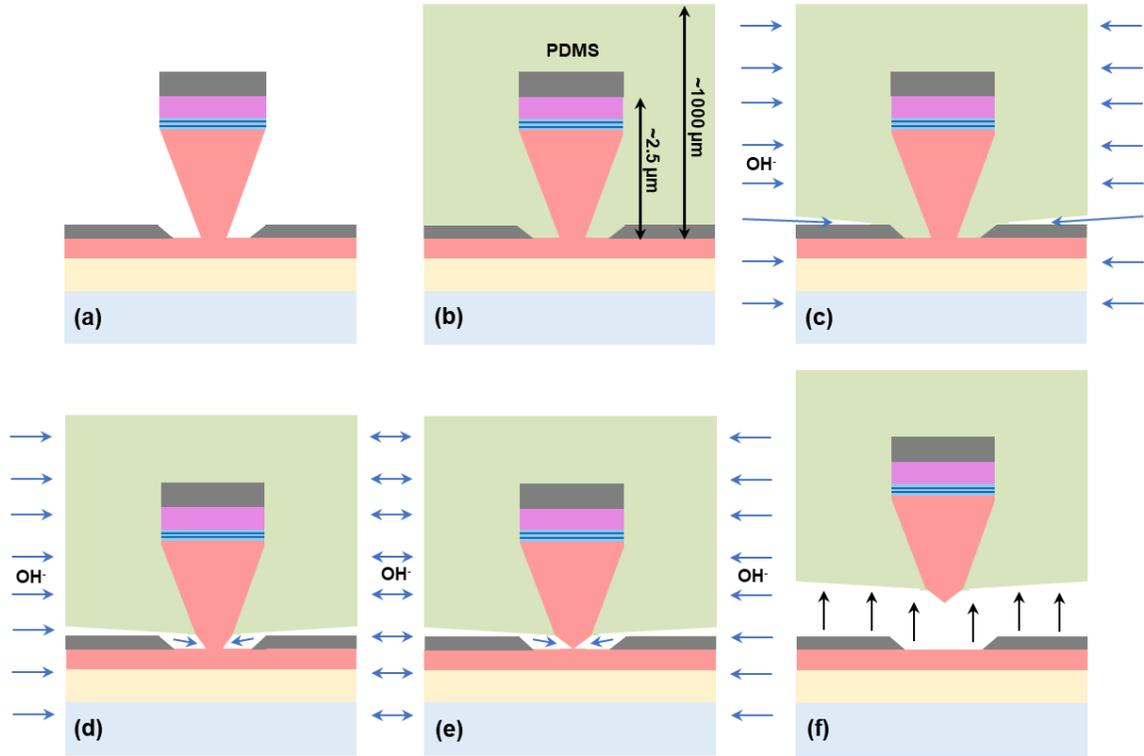
Figure 4.2.4: Cross sectional schematic of the nanowire removal process. (a) Directional Ni deposition. (b) PDMS coating. (c-e) Extended duration room temperature KOH etching. (f) Liftoff of nanowire embedded in PDMS.
