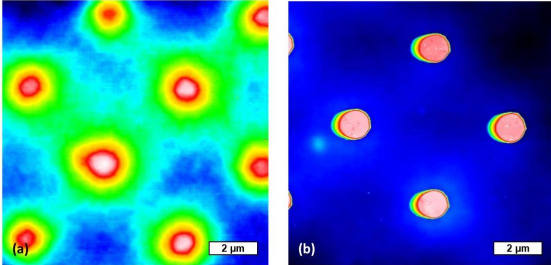
Figure 3.8.2: AFM maps of a nanowire sample before (a) and after (b) the nanowires tips are exposed by etching back the PDMS.
