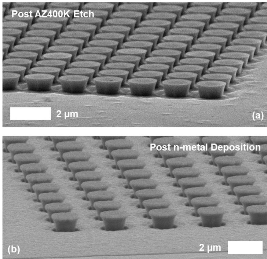
Figure 4.5.7: SEM images of 1.5  $\mu\text{m}$  micropillars on a 2  $\mu\text{m}$  pitch following AZ400K etching (a), and 1.25  $\mu\text{m}$  micropillars on a 2.5  $\mu\text{m}$  pitch following deposition of the 40 nm Ni p-contact and 30/100 nm Cr/Au n-contact (b).
