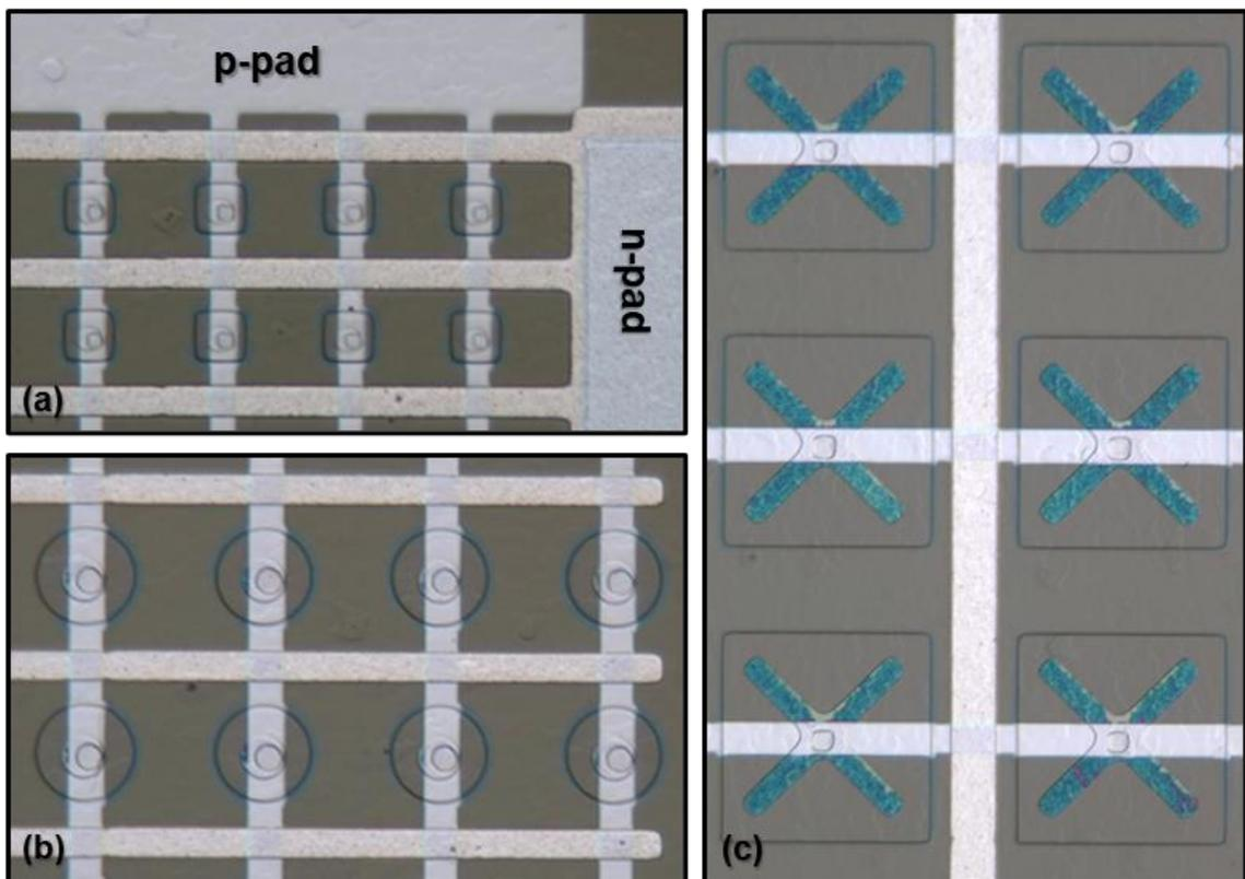
Figure 4.4.5: Optical images of 10  $\mu\text{m}$  (a) 30  $\mu\text{m}$  (b), and 50  $\mu\text{m}$  (c)  $\mu\text{LEDs}$ . (a) shows the locations of the p- and n-contact pads as well as the location of the contact open over the n-pad. Discoloration of the annealed p-contact metal can be seen in (c).
