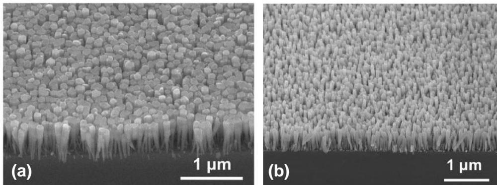
Figure 2.2.2: SEM images of epitaxial AlGaN nanowires grown using MBE (a) [58] and MOCVD (b) [66]. Reprinted with permission [58, 66].
