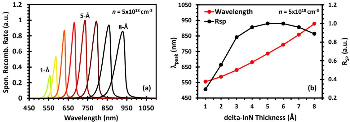
Figure 5.1.3: (a) Spontaneous recombination rate spectra for  $\text{In}_{0.15}\text{Ga}_{0.85}\text{N}/\text{In}_{0.3}\text{Ga}_{0.7}\text{N}/\text{delta-InN}$  structures of varying delta-InN thickness for  $n = 5 \times 10^{18} \text{ cm}^{-3}$ . (b)  $\lambda_{\text{peak}}$  and  $R_{sp}$  as a function of delta-InN thickness.
