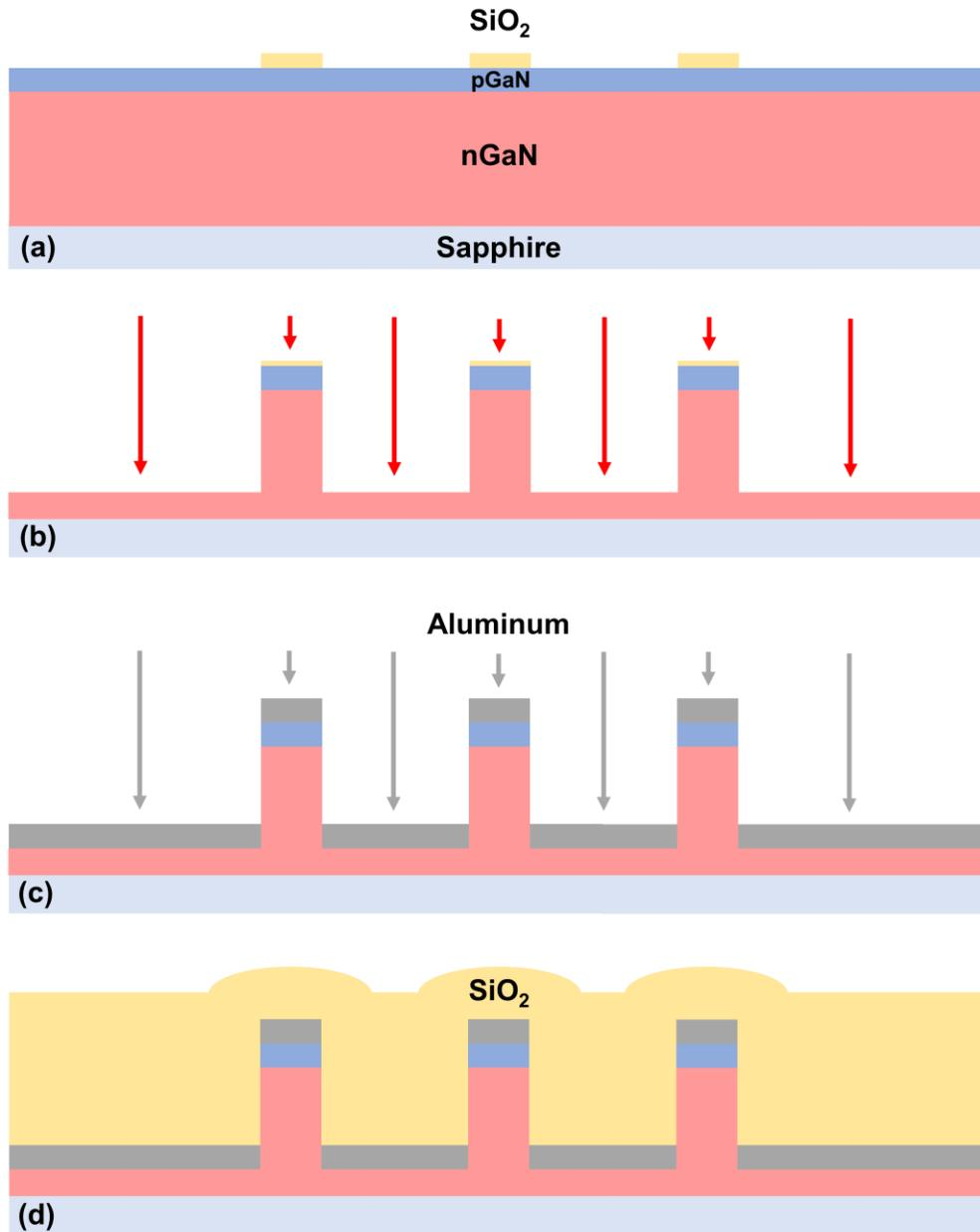
Figure 4.6.1(a-d): Deposition and patterning of  $\text{SiO}_2$  to form an etch mask (a), Cl etching of the AlGaN to form nanowires (b), directional Al deposition (c), conformal  $\text{SiO}_2$  deposition (d).
