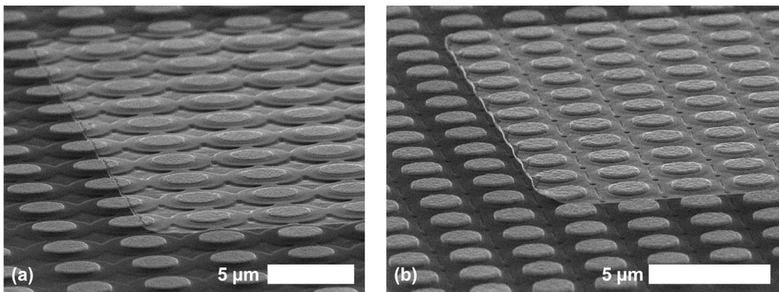
Figure 4.5.15: SEM images of reduced size arrays following conformal Ni deposition. The diameter/pitches of the arrays shown in (a) and (b) are 2.5/4.5 μm and 2/3.5 μm respectively.
