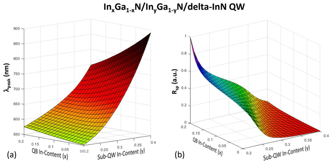
Figure 5.1.4: (a)  $\lambda_{\text{peak}}$  dependence on the In-content of the QB and sub-QW regions for an  $\text{In}_x\text{Ga}_{1-x}\text{N}/\text{In}_y\text{Ga}_{1-y}\text{N}/\text{delta-InN}$  QW with a 3 Å delta-layer, showing that red emission wavelength is continuously tunable through small variations of the In-content in these regions. Chart colors are accurate. (b)  $R_{\text{sp}}$  dependence on the In-content in the QB and sub-QW regions.
