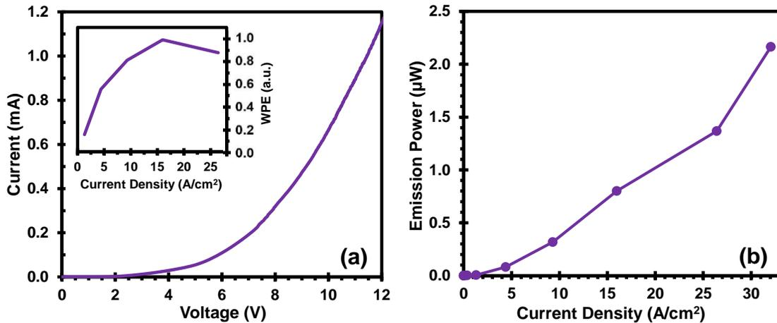
Figure 4.1.7: (a) Linear I-V characteristics of a 30x30 nanowire array LED, showing a  $V_{th}$  of approximately 7 V. The inset shows the normalized WPE of the LED, with peak WPE occurring at 16 A/cm<sup>2</sup> and minimal efficiency droop at higher current densities. (b) Emission power as a function of current density.
