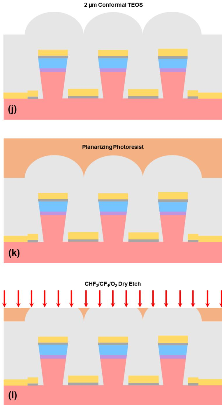
Figure 4.5.6(j-l): PECVD deposition of 2  $\mu\text{m}$  of conformal TEOS (j), coating of a semi-self-planarizing photoresist layer onto the TEOS surface (k), planarization of the TEOS surface using a F dry etch (l).
