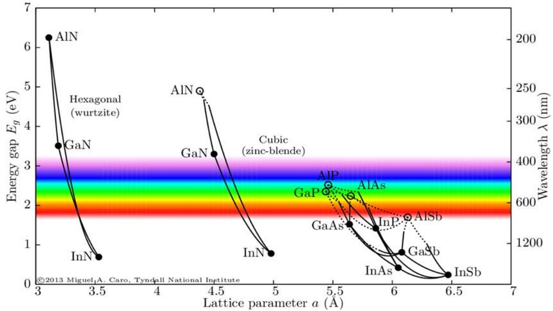
Figure 1.4.1: Bandgap vs lattice parameter for III-V semiconductors and their alloys [19].
