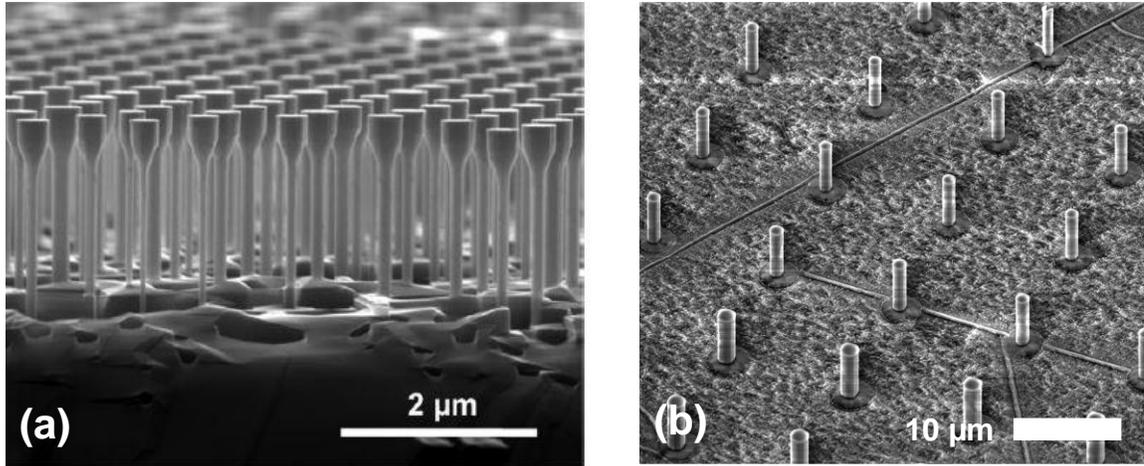
Figure 2.2.4: SEM images showing top-down fabrication GaN nanowires (a) [70] and AlGaN nanowires fabricated in the SMFL (b). Reprinted with permission [70].
