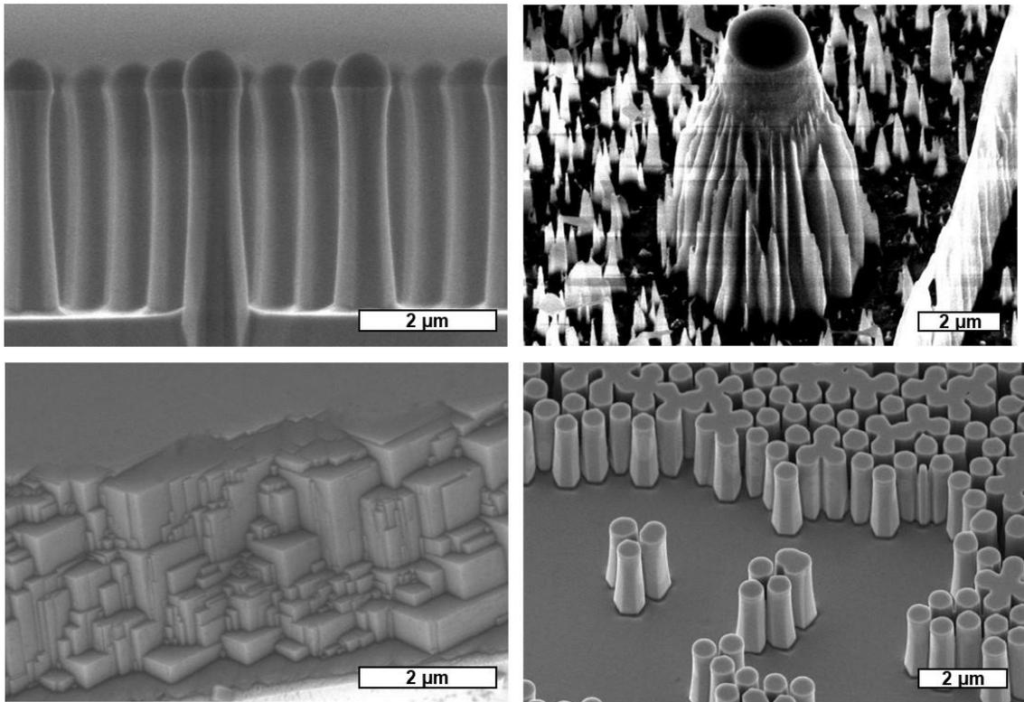
Figure 3.8.1: Off-normal SEM images of various GaN structures.
