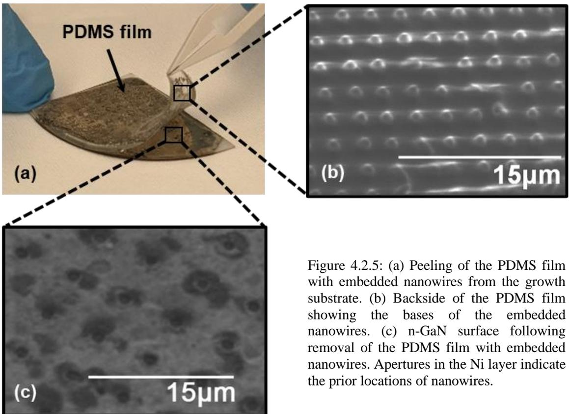
Figure 4.2.5: (a) Peeling of the PDMS film with embedded nanowires from the growth substrate. (b) Backside of the PDMS film showing the bases of the embedded nanowires. (c) n-GaN surface following removal of the PDMS film with embedded nanowires. Apertures in the Ni layer indicate the prior locations of nanowires.
