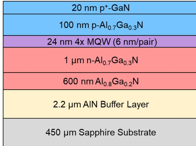
Figure 4.5.5: Cross-sectional representation of the AlGaN-delta-GaN epitaxy used during process development.
