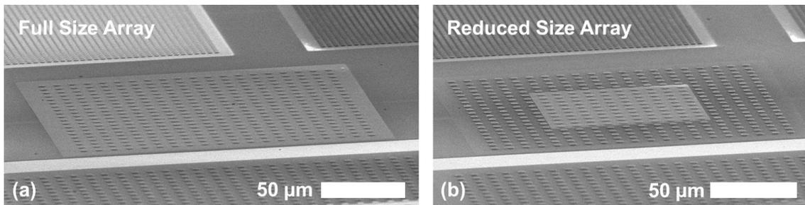
Figure 4.5.14: SEM images of completed full size (a) and reduced size (b) devices following deposition of 25 nm of conformal Ni to connect many micropillars in parallel.
