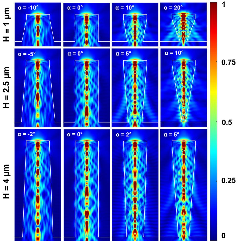
Figure 4.3.4: Cross-sectional electric field intensity plots for 1  $\mu\text{m}$ , 2.5  $\mu\text{m}$ , and 4  $\mu\text{m}$  tall structures with diameters of 1  $\mu\text{m}$  and taper angles between  $-10^\circ$  and  $20^\circ$  for TE-polarized emission at  $\lambda = 270 \text{ nm}$ .
