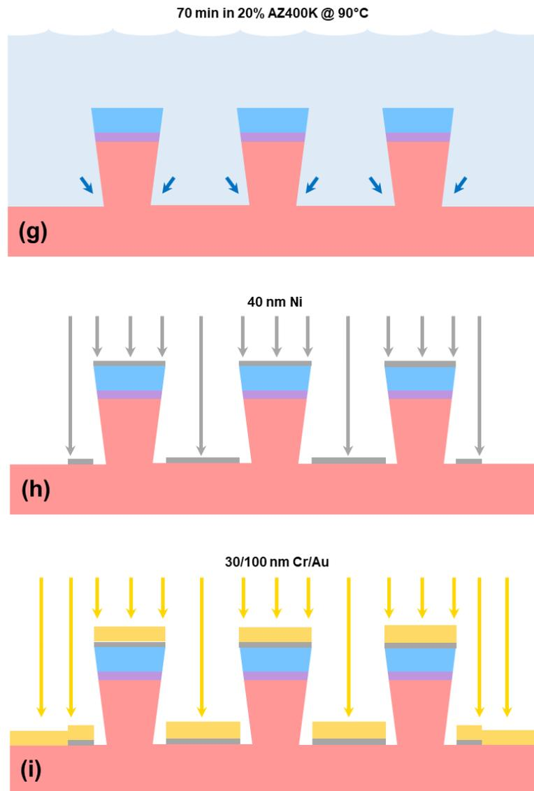
Figure 4.5.6(g-i): Extended wet etching of the AlGaN for 70 min in 20% AZ400K to produce an inverse taper sidewall profile (g), deposition of 40 nm Ni on top of the micropillars followed by annealing in O<sub>2</sub> at 550°C to form an ohmic p-contact (h), deposition of 30/100 nm Cr/Au to form an unannealed ohmic n-contact to the n-AlGaN (i).
