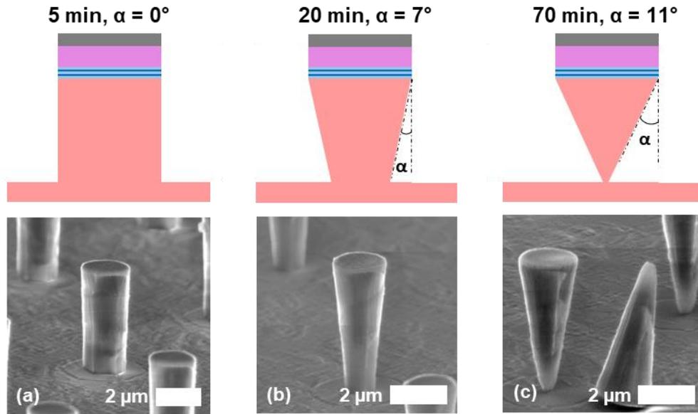
Figure 4.2.2: Nanowires with 2  $\mu\text{m}$  top diameters following 5, 20, and 70 min of KOH etching, with taper angles of  $0^\circ$ ,  $7^\circ$ , and  $11^\circ$  respectively.
