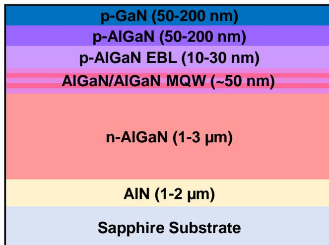
Figure 3.2.1: Representative DUV LED epitaxial stack grown either by MOCVD or MBE (not to scale).
