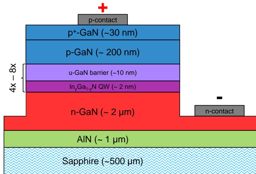
Figure 1.1.3: Representative structure of modern blue LED. Layer thicknesses are approximate and shown layer thicknesses are not to scale.
