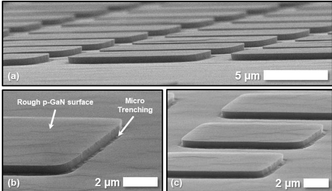
Figure 4.4.3: SEM images of 10  $\mu\text{m}$   $\mu\text{LED}$  mesas taken at  $85^\circ$  (a) and  $80^\circ$  (b,c) off normal. Roughness of the p-GaN surface and micro-trenching are highlighted in (b).
