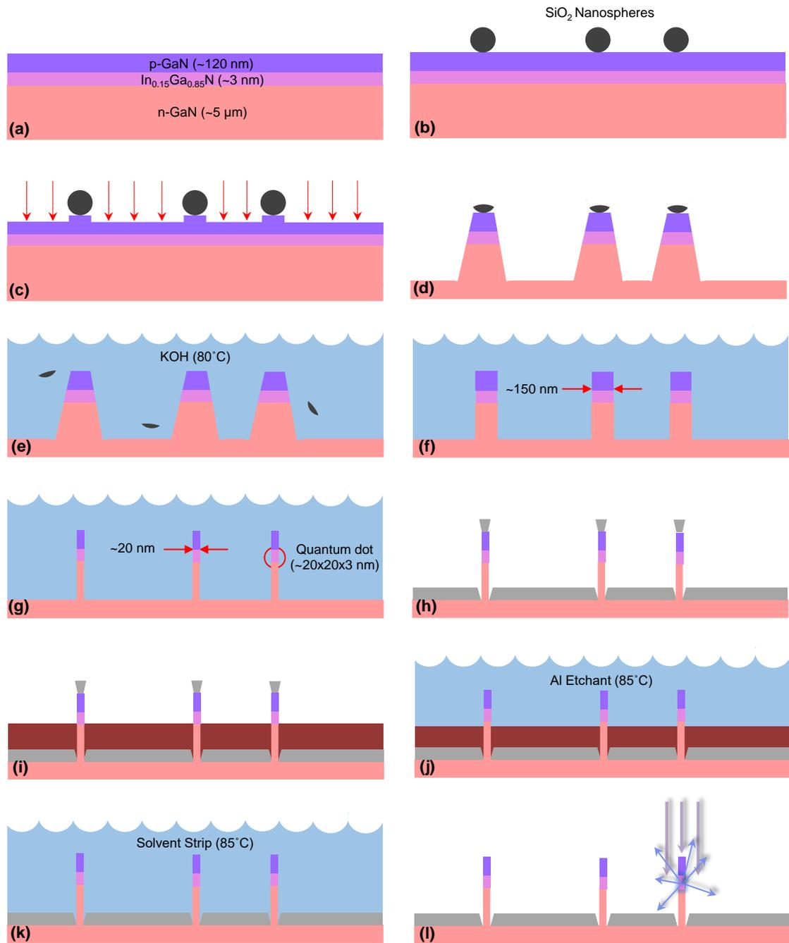
Figure 5.4.1: Nanowire QD SPE fabrication schematic (not to scale).
