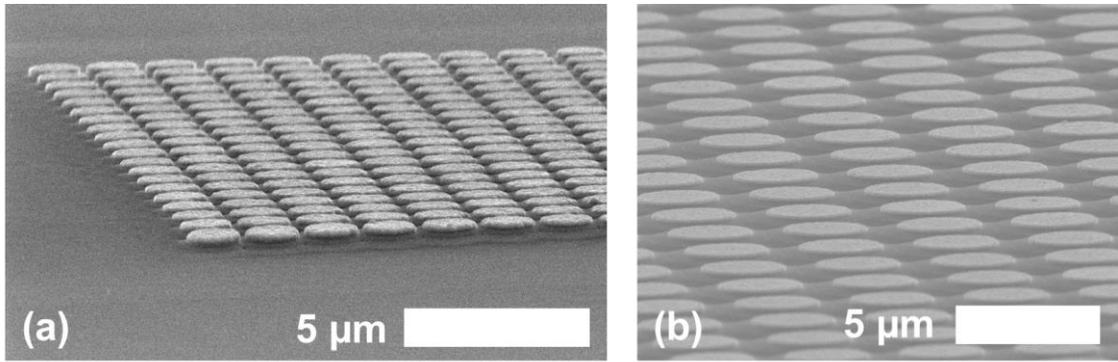
Figure 4.5.12: SEM images showing the Cr/Au covered surfaces of micropillars following successful etchback of the TEOS.
