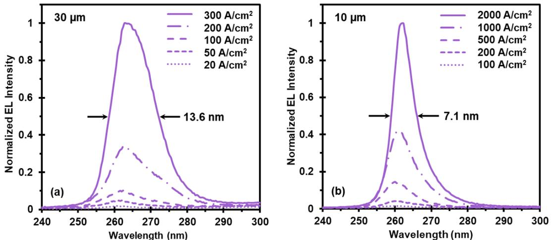
Figure 4.4.7: Normalized EL spectra for individual 30  $\mu$ m (a) and 10  $\mu$ m (b)  $\mu$ LEDs at various current densities. Emission peaks for 30  $\mu$ m and 10  $\mu$ m devices at their maximum measured current densities were located at 264.3 nm and 262 nm respectively. Emission linewidths at maximum measured current densities were 13.6 nm and 7.1 nm respectively.
