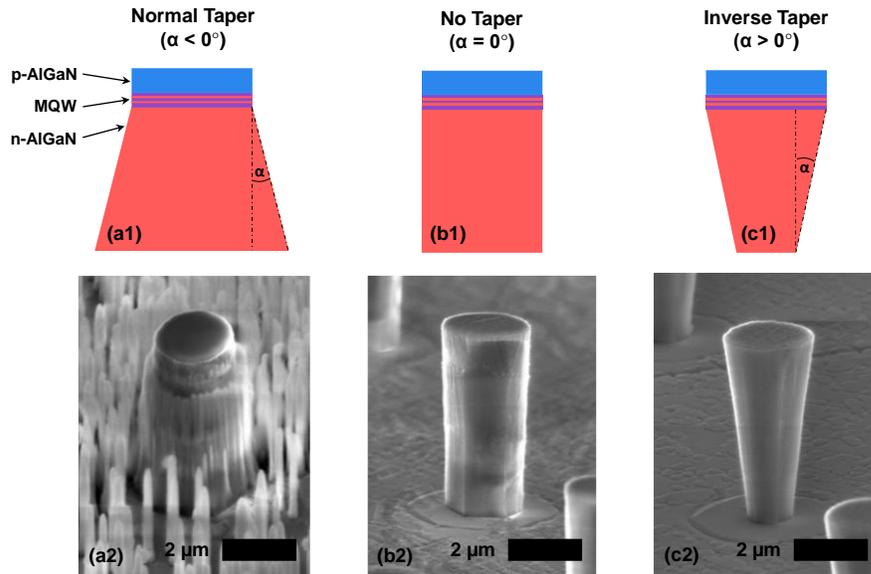
Figure 4.3.1: Cross sectional schematics showing structures with normal taper (a1), no taper (b1), and inverse taper (c1), along with representative SEM images of each structure (a2-c2).
