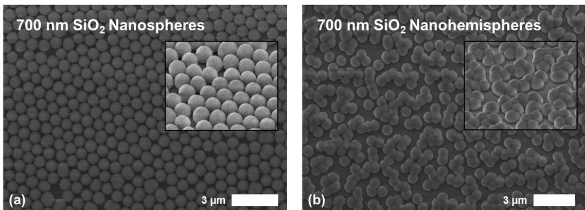
Figure 5.5.7: SEM images of 700 nm SiO<sub>2</sub> nanosphere (a) and nanohemisphere (b) arrays, formed through spin-coating of aqueous nanosphere solutions and subsequent RIE and PECVD SiO<sub>2</sub> deposition in the case of (b). Insets show the sample surfaces at 45°.
