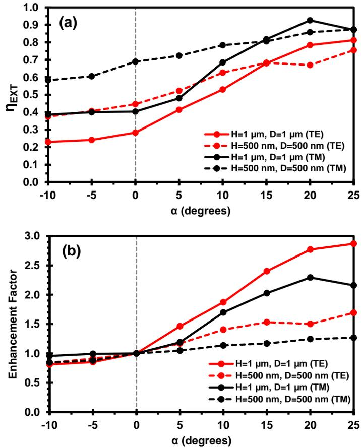
Figure 4.3.9:  $\eta_{\text{EXT}}$  (a) and  $\eta_{\text{EXT}}$  enhancement factor (b) for TE (red) and TM (black) polarizations as a function of taper angle  $\alpha$  for  $1 \mu\text{m}$  tall,  $1 \mu\text{m}$  diameter structures (solid), and  $500 \text{ nm}$  tall,  $500 \text{ nm}$  diameter structures (dashed) at  $\lambda = 270 \text{ nm}$ . Both structures have ARs of 1 (height/diameter).
