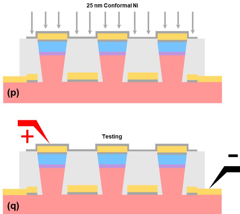
Figure 4.5.6(p-q): Conformal deposition of Ni to form to connect each array of micropillars in parallel (p), testing of a completed device (q).
