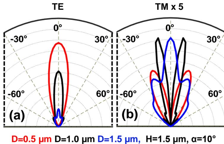
Figure 4.3.8: Far-field emission patterns for TE-polarized (a) and TM-polarized (b) light for 0.5  $\mu\text{m}$ , 1  $\mu\text{m}$ , and 1.5  $\mu\text{m}$  diameter structures with a height at 1.5  $\mu\text{m}$  and a taper angle of 10° at  $\lambda = 270 \text{ nm}$ . TM-polarized emission (b) is multiplied by a factor of 5 to better show the emission pattern.
