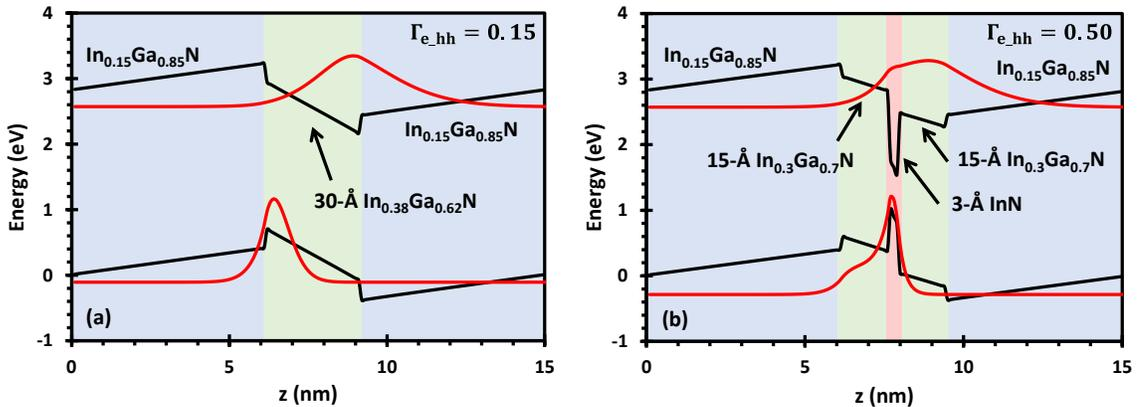
Figure 5.1.1: Bandstructures and ground state wavefunctions in an  $\text{In}_{0.15}\text{Ga}_{0.85}\text{N}/\text{In}_{0.38}\text{Ga}_{0.62}\text{N}$  QW (a) and an  $\text{In}_{0.15}\text{Ga}_{0.85}\text{N}/\text{In}_{0.3}\text{Ga}_{0.7}\text{N}/\text{delta-InN}$  QW with a 3 nm delta-layer (b), showing enhanced  $\Gamma_{e\_hh}$  for the delta-InN structure.
