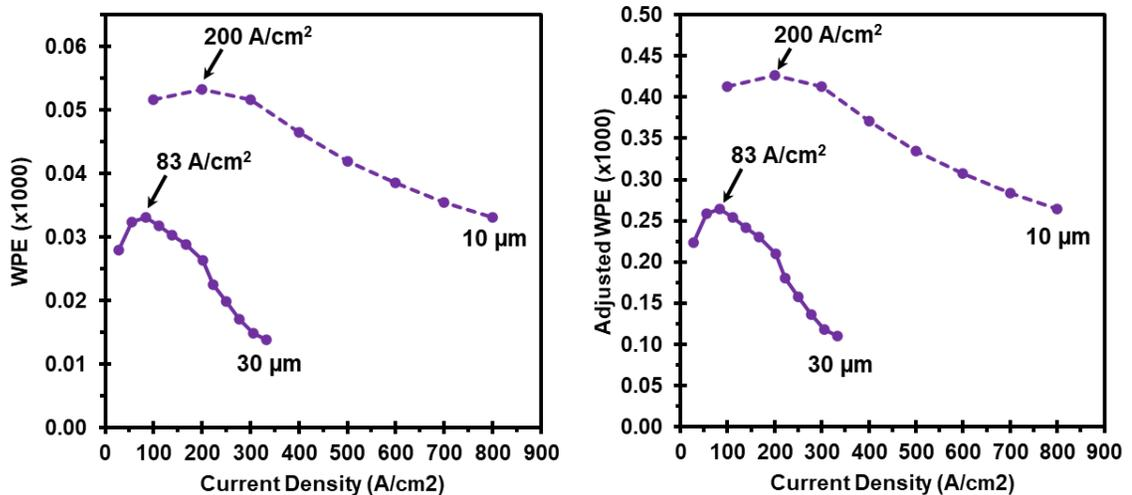
Figure 4.4.11: Measured (a) and adjusted (b) wall plug efficiency as a function of current density for 10 μm (dashed) and 30 μm (solid) μLEDs. The onset of efficiency droop was found to occur at 200 A/cm<sup>2</sup> for 10 μm devices and at 83 A/cm<sup>2</sup> for 30 μm devices. A WPE value of 1.0 is equal to 100% efficiency.
