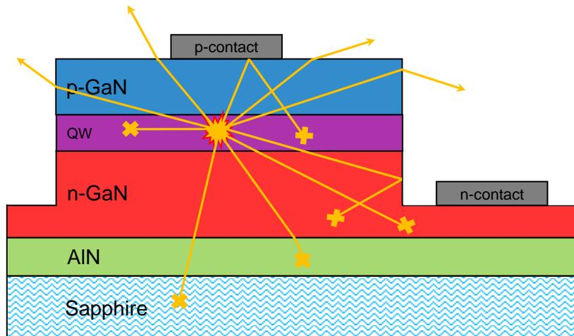
Figure 1.1.5: Light extraction from a simplified LED structure. Ten photons are emitted from a point-source in the center of the active region, with lines terminating in arrows representing escaping photons, and lines terminating in X's representing photons reabsorbed by the structure.
