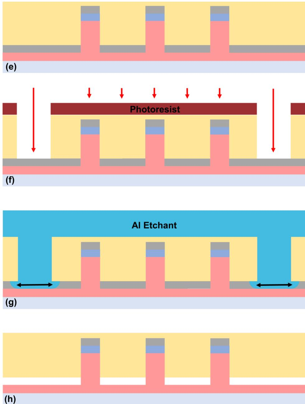
Figure 4.6.1(e-h): SiO<sub>2</sub> planarization (e), opening of apertures in the SiO<sub>2</sub> layer (f), removal of the Al layer under the SiO<sub>2</sub> using an Al wet etch (g-h).
