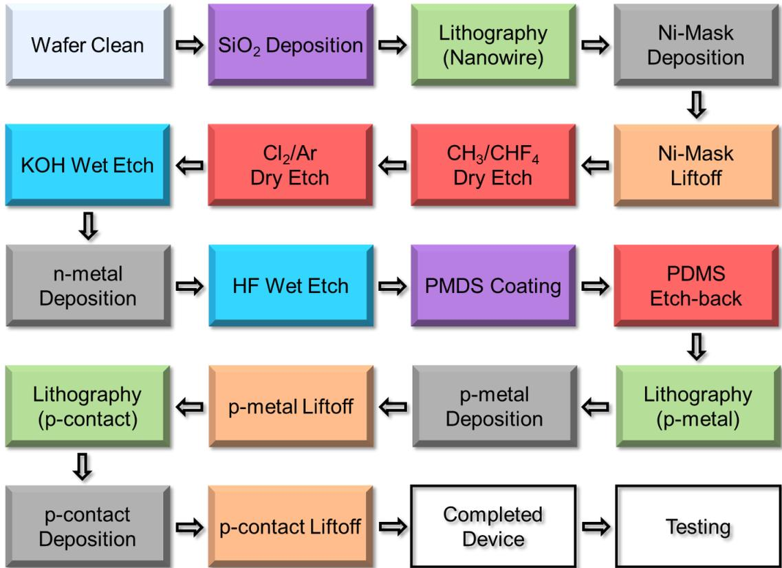
Figure 3.1.3: Nanowire LED fabrication process flow with color coded process steps.
