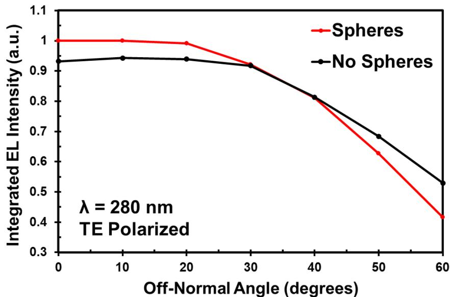
Figure 5.5.9: Angle-dependent EL data for 700 nm nanospheres, showing a clear increase in emission intensity at low angles less than 30° for samples with nanospheres when compared to samples with no nanospheres.
