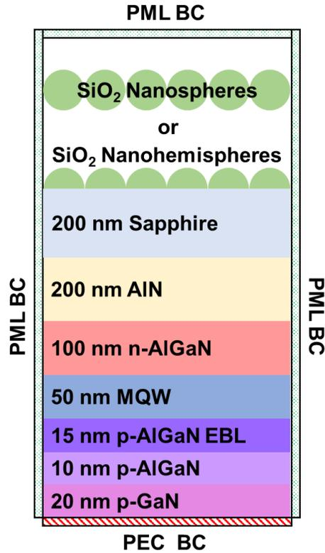
Figure 5.5.1: Cross-sectional representation of the three-dimensional structure used for FDTD simulation. Perfectly matched layer (PML) and perfect electric conductor (PEC) boundary conditions (BC) are shown at the domain surfaces.
