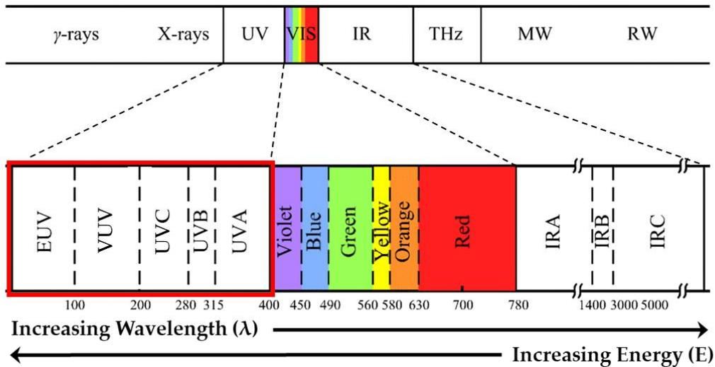
Figure 1.2.1: Electromagnetic spectrum between 10 and 1000 nm, showing the wavelength ranges of V-UV, UV-C, UV-B, and UV-A light.
