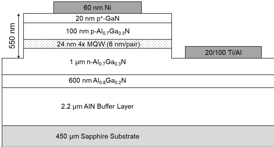
Figure 4.4.2: Not-to-scale cross sectional representation of a completed  $\mu$ LED device.
