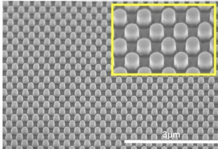
Figure 2.1.3: An SEM image of a photonic crystal fabricated in AlGaN using a combination of wet and dry etching. Reprinted with permission [23].
