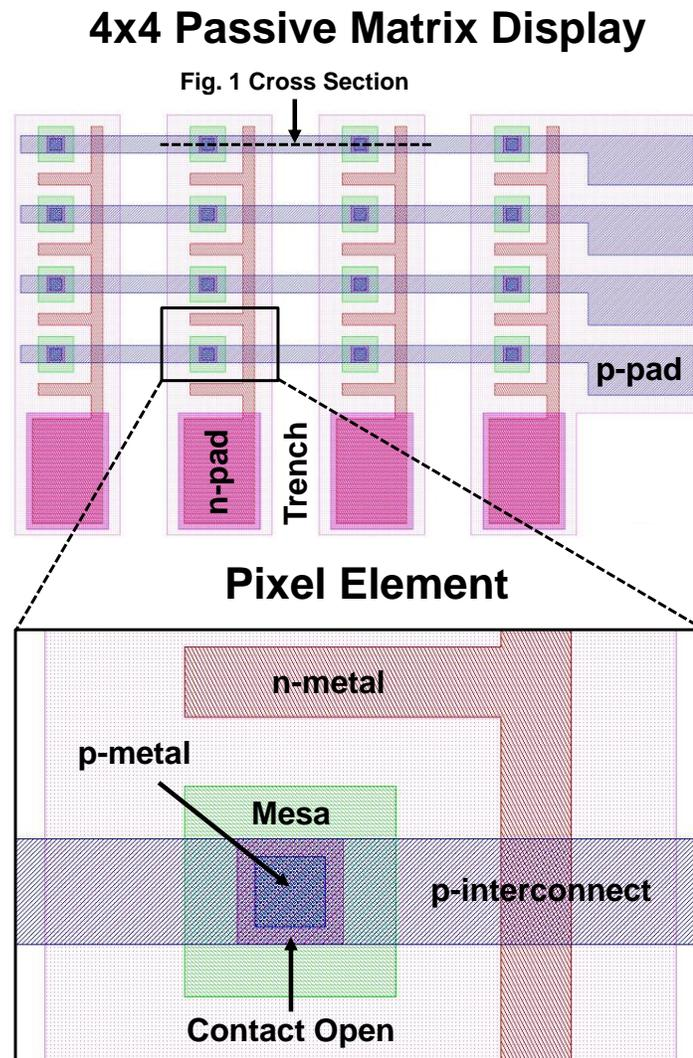
Figure 5.3.2: Layout view of a 4x4 passive matrix array (top) and an enlarged view of a single pixel element of the display (bottom). The location of the cross section described in Figure 5.3.1 is shown in the top center of the 4x4 display at top.
