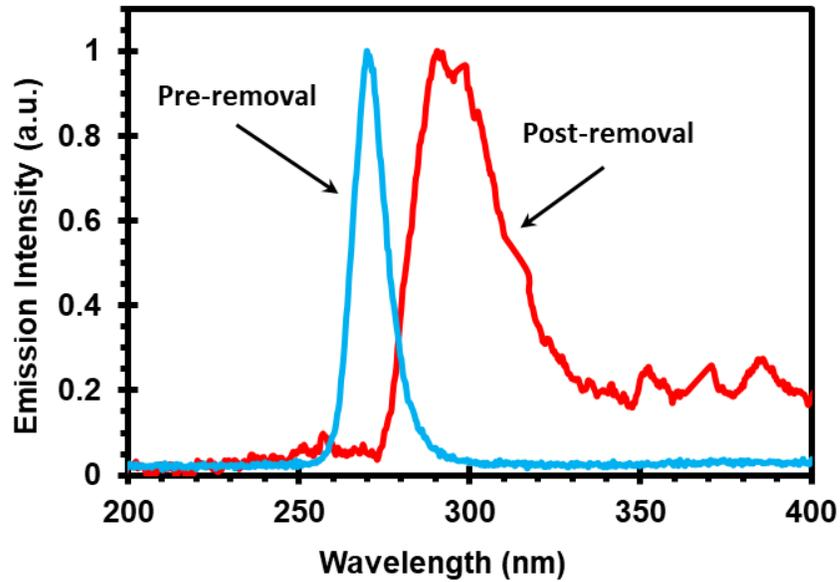
Figure 4.2.6: PL emission spectrums of the bulk epi (blue) and the nanowires embedded in the PDMS film (red). The pre- and post-removal curves have peaks at 267 nm and 292 nm respectively.
