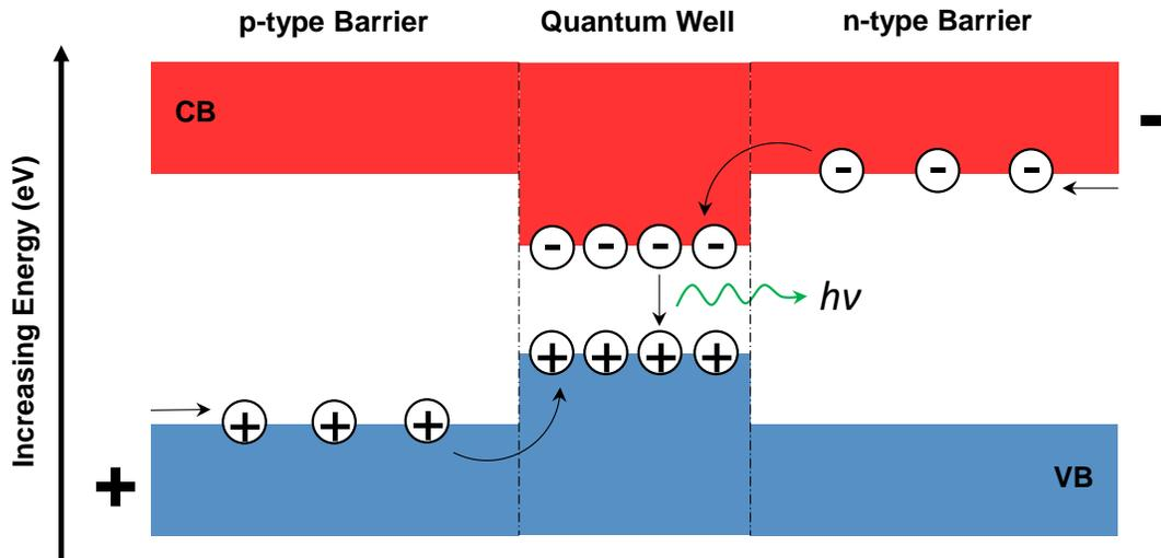
Figure 1.1.2: Electron-hole recombination in a generic PN quantum well. Band bending is not shown for simplicity.
