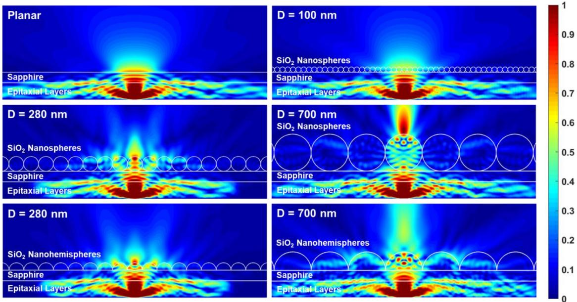
Figure 5.5.3: Cross-sectional electric field intensities for simulation structures of variable nanosphere and nanohemisphere diameters, showing spatial variation in electric field intensities with nanostructure diameter.
