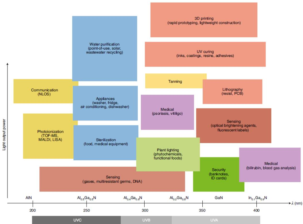
Figure 1.3.1: Applications of ultraviolet light categorized by wavelength and output power. Reprinted with permission [13].
