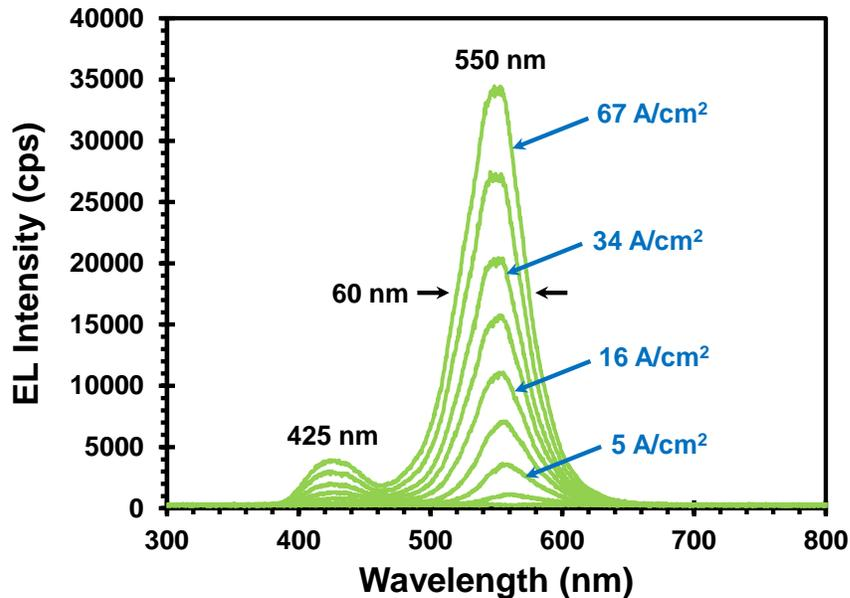
Figure 5.2.3: EL spectra of a micropillar array LED at various current densities, showing a peak emission wavelength of ~550 nm and a linewidth of ~60 nm.
