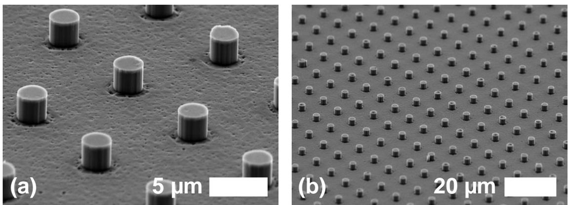
Figure 5.2.2: SEM images show the nanowire arrays after the hydroxyl-based wet etch step.
