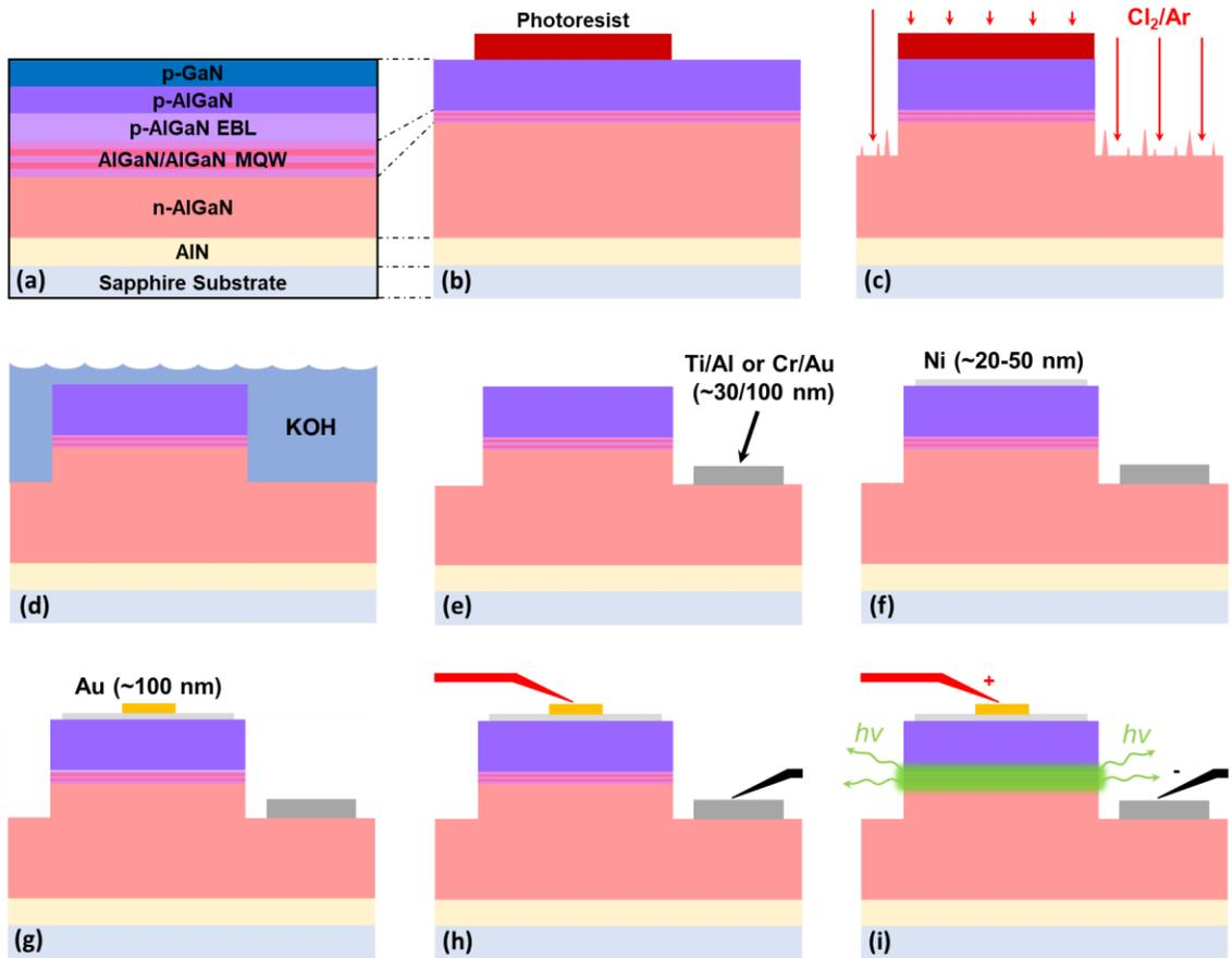
Figure 3.1.2: Mesa LED fabrication schematic showing mesa etching and metallization steps (not to scale).
