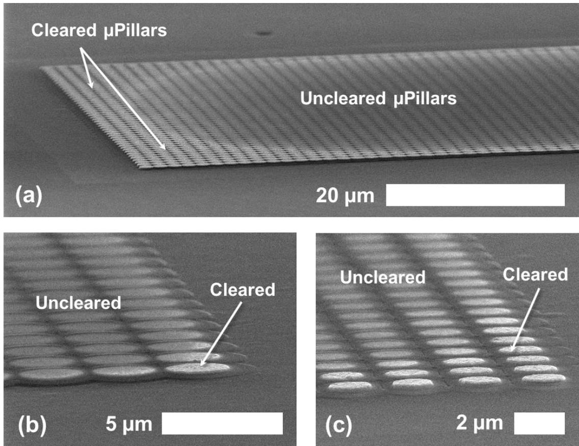
Figure 4.5.13: SEM images highlighting the issues which can occur during planarization of TEOS over isolated arrays of micropillars. (a) shows a large, dense array in which the corner regions have cleared to expose the Cr/Au on the micropillars, while the center of the array remains covered in TEOS. Likewise (b) and (c) show close up images of the corner regions of similar arrays.
