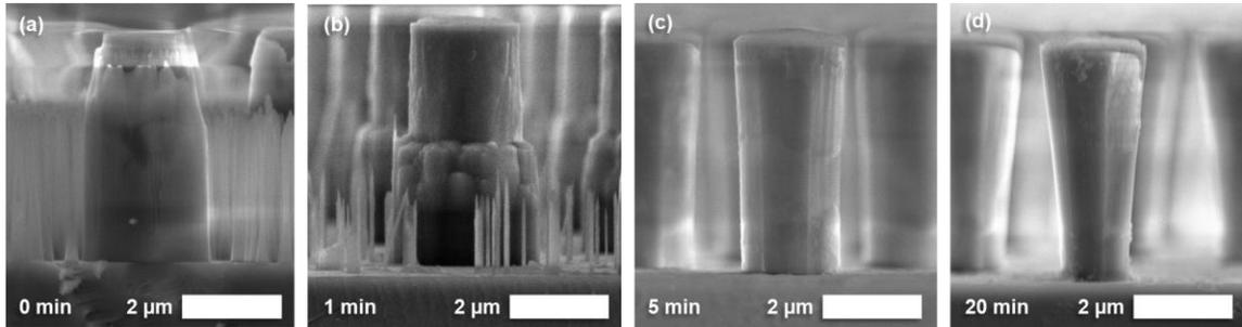
Figure 4.1.3: SEM images showing AlGaIn nanowires at various points in the fabrication process. Nanowires after dry etch (a), and 1 min (b), 5 min (c), and 20 min (d) in 0.8 wt.% aqueous KOH at 80°C.
