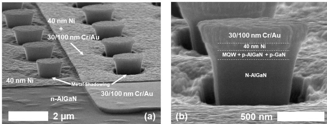
Figure 4.5.9: SEM images showing the intersection between regions of exposed n-AlGaN, annealed Ni, and Cr/Au on annealed Ni (a), and a near cross sectional view of an 800 nm micropillar covered with 40 nm Ni and 30/100 nm Cr/Au (b).
