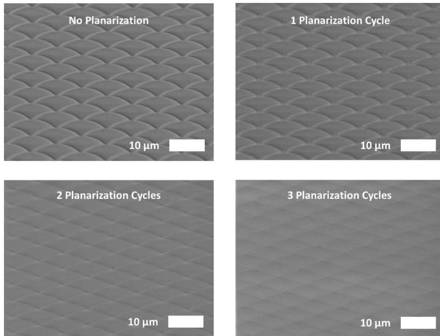
Figure 3.7.3: SEM images of micropillars (2.5  $\mu\text{m}$  diameter, 2  $\mu\text{m}$  height, 10  $\mu\text{m}$  pitch) after 0 planarization cycles,  $h = 1.62 \mu\text{m}$  (a), 1 planarization cycle,  $h = 610 \text{ nm}$  (b), 2 planarization cycles,  $h = 76 \text{ nm}$  (c), and 3 planarization cycles,  $h = 24 \text{ nm}$  (d) [18].
