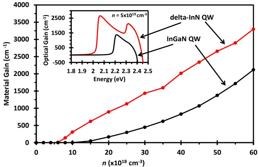
Figure 5.1.6: Material gain as a function of  $n$  for an  $\text{In}_{0.15}\text{Ga}_{0.85}\text{N}/\text{In}_{0.38}\text{Ga}_{0.62}\text{N}$  QW (black) and an  $\text{In}_{0.15}\text{Ga}_{0.85}\text{N}/\text{In}_{0.3}\text{Ga}_{0.7}\text{N}/\text{delta-InN}$  QW (red). Inset shows the optical gain spectra at  $n = 5 \times 10^{18} \text{ cm}^{-3}$ .
