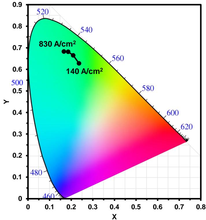
Figure 5.3.8: CIE 1931 coordinates of 60  $\mu\text{m}$  devices driven between 140  $\text{A}/\text{cm}^2$  and 830  $\text{A}/\text{cm}^2$ .
