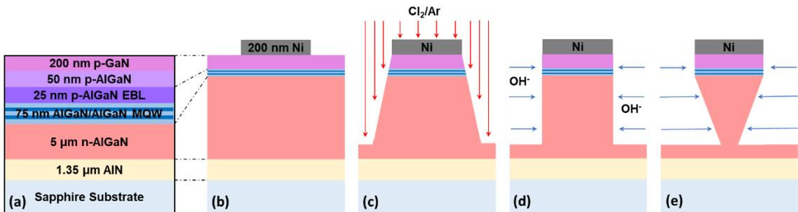
Figure 4.2.1: (a) Simplified DUV LED epitaxial layer stack (not to scale). Nanowire formation process showing (b) deposition of the Ni hard mask, (c) the  $\text{Cl}_2/\text{Ar}$  dry etch, (d) 5 min of wet etching in 40% AZ400K at  $80^\circ\text{C}$ , and (e) 70 min of wet etching in 40% AZ400K at  $80^\circ\text{C}$ .
