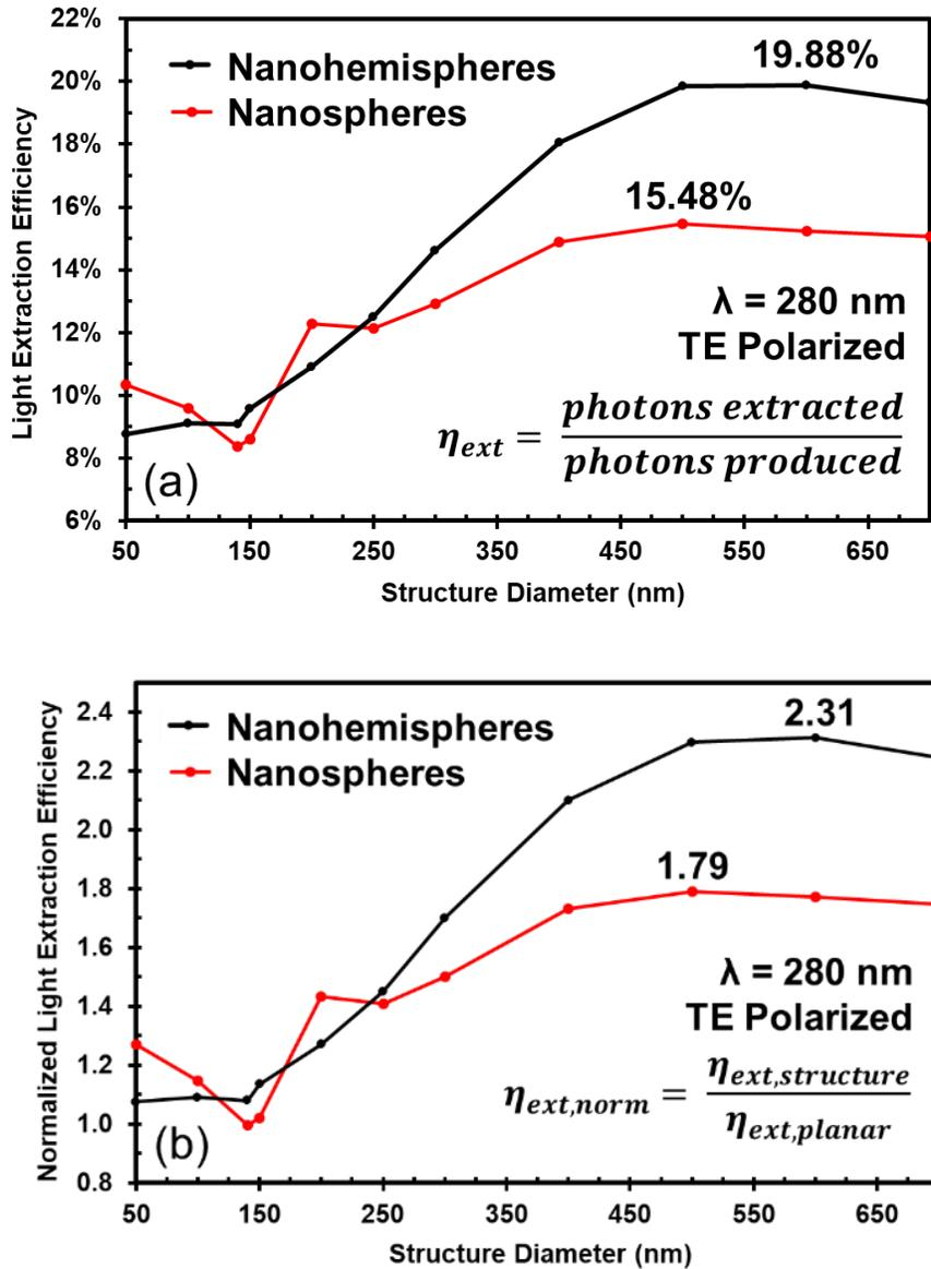
Figure 5.5.2: (a)  $\eta_{EXT}$  of SiO<sub>2</sub> nanospheres and nanohemispheres of variable diameter. (b) Normalized  $\eta_{EXT}$ s of SiO<sub>2</sub> nanospheres and nanohemispheres calculated by dividing the values shown in (a) by the  $\eta_{EXT}$  of a planar sapphire structure with no SiO<sub>2</sub> nanostructures (8.57%).
