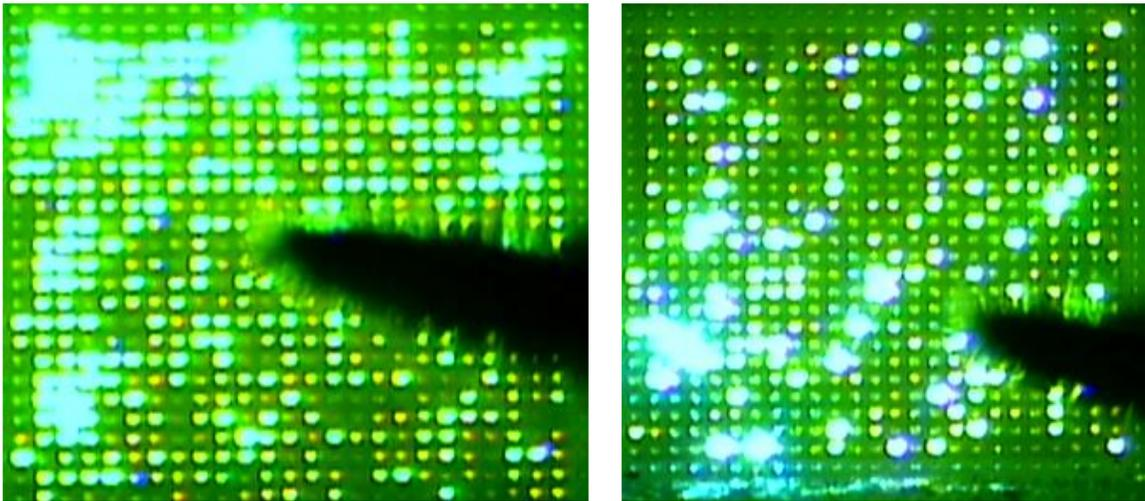
Figure 5.2.4: Optical images of the illuminated nanowire arrays taken using a microscope camera.
