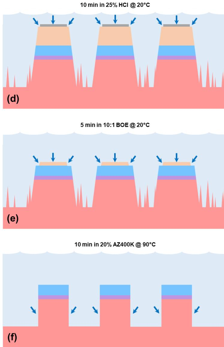
Figure 4.5.6(d-f): Wet etching of the Ni mask in 25% HCl (d), wet etching of the underlying TEOS in 10:1 BOE (e), etching of the AlGaIn for 10 min in 20% AZ400K to remove etch grass and straighten sidewalls (f).
