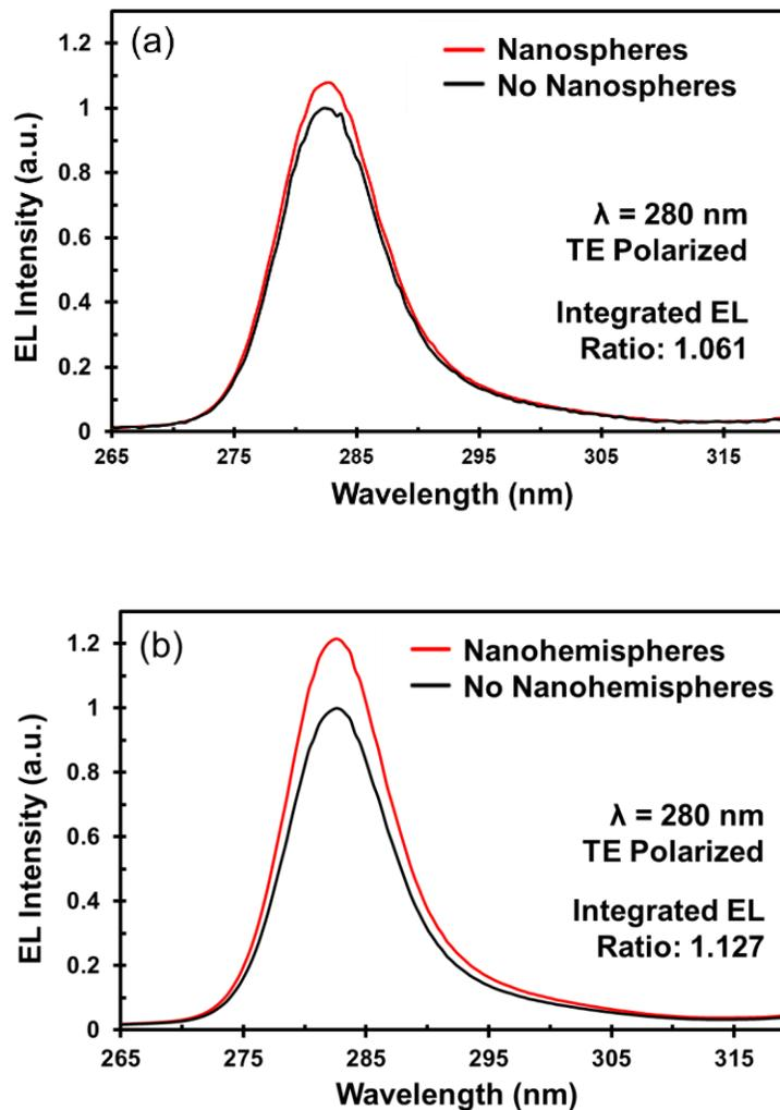
Figure 5.5.8: EL spectra for 700 nm nanospheres (a) and nanohemispheres (b) plotted taken at normal incidence between 260 nm and 315 nm. The much larger  $\eta_{\text{EXT}}$  enhancement of the nanohemisphere array is evidenced by the larger variation in the maxima of the curves for samples with and without nanohemispheres.
