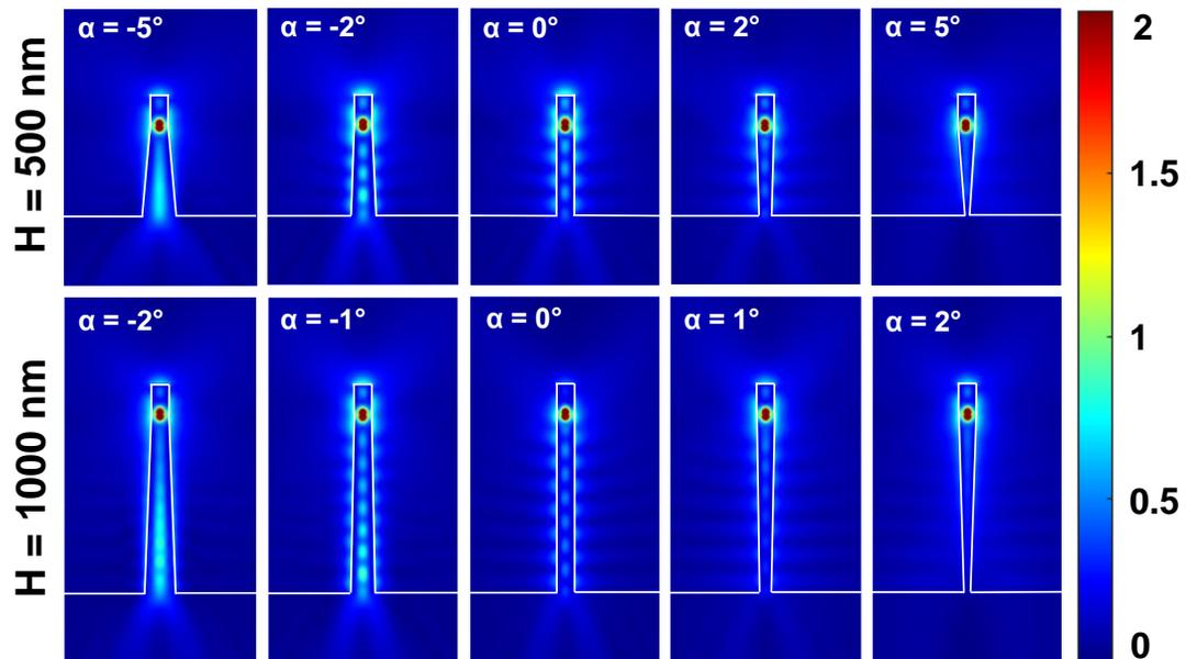
Figure 4.3.11: Cross-sectional electric field intensity plots for 500 nm and 1000 nm tall structures with diameters of 100 nm and taper angles between  $-5^\circ$  and  $5^\circ$  for TE-polarized (top) and TM-polarized (bottom) emission at  $\lambda = 270$  nm. Field intensity is halved in comparison to Figures 4, 5, and 12 to ensure cavity modes can be seen.
