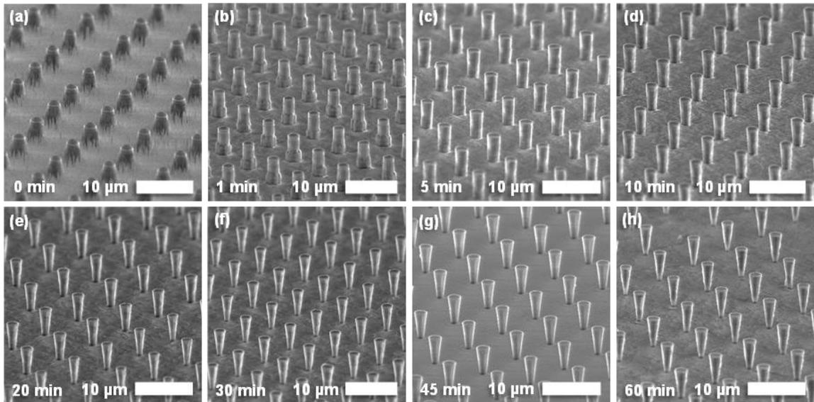
Figure 4.1.2: SEM images showing AlGaN nanowires at various points in the fabrication process. Nanowires after dry etch (a), and 1 min (b), 5 min (c), 10 min (d), 20 min (e), 30 min (f), 45 min (g), and 60 min (h) in 0.8 wt.% aqueous KOH at  $80^\circ\text{C}$ .
