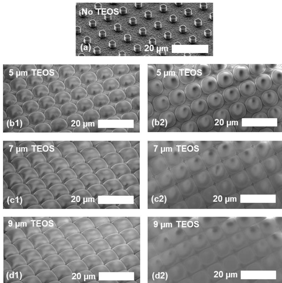
Figure 4.5.1: SEM images showing micropillars (2  $\mu\text{m}$  diameter, 2  $\mu\text{m}$  height, 10  $\mu\text{m}$  pitch) following dry etching and KOH treatment (a), and subsequently after 5  $\mu\text{m}$  (b), 7  $\mu\text{m}$  (c), and 9  $\mu\text{m}$  (d) of conformal TEOS deposition. Images a, b1, c1, and d1 were taken at 45° off normal, while b2, c2, and d2 were taken normal to the sample surface [104].
