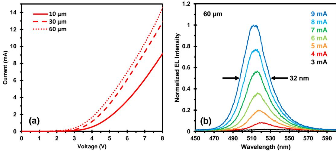
Figure 5.3.6: (a) Current voltage characteristics for 10, 30, and 60  $\mu\text{m}$   $\mu\text{LEDs}$ . (b) Electroluminescence spectra of a 60  $\mu\text{m}$   $\mu\text{LED}$  driven at between 1 mA and 9 mA, showing peak emission at  $\sim 515$  nm and a FWHM of  $\sim 32$  nm.
