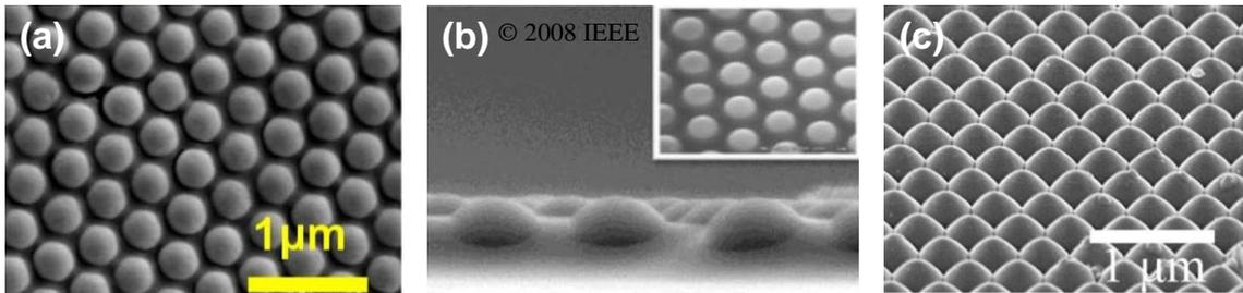
Figure 2.1.4: SEM images showing SiO<sub>2</sub>/PS microlens arrays (a-b) [35,36] and nanostructured AlGaIn (c) [44]. Reprinted with permission [35, 36, 44] © Optical Society of America, © IEEE.
