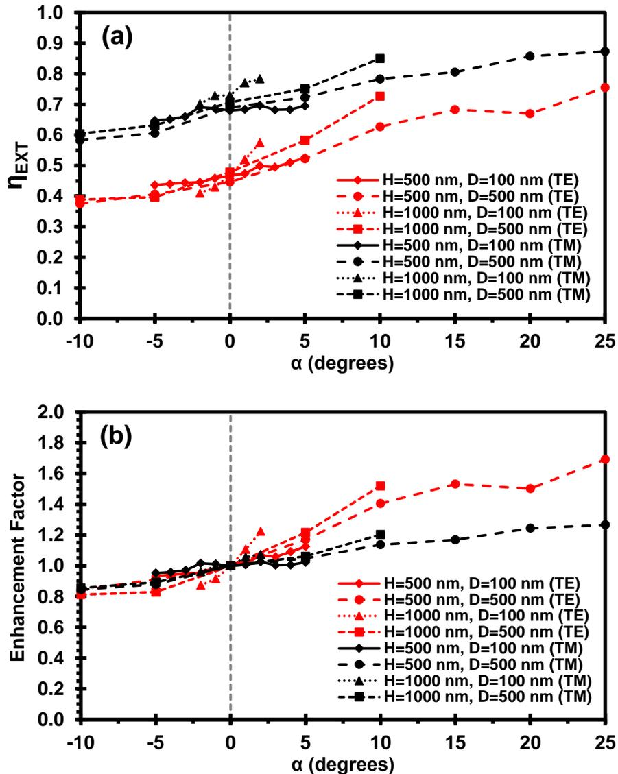
Figure 4.3.10:  $\eta_{EXT}$  (a) and  $\eta_{EXT}$  enhancement factor (b) for TE (red) and TM (black) polarizations as a function of taper angle  $\alpha$  for 500/100 nm tall/diameter (diamond), 500/500 nm (circle), 1000/100 nm (triangle), and 1000/500 nm (square) structures at  $\lambda = 270$  nm.
