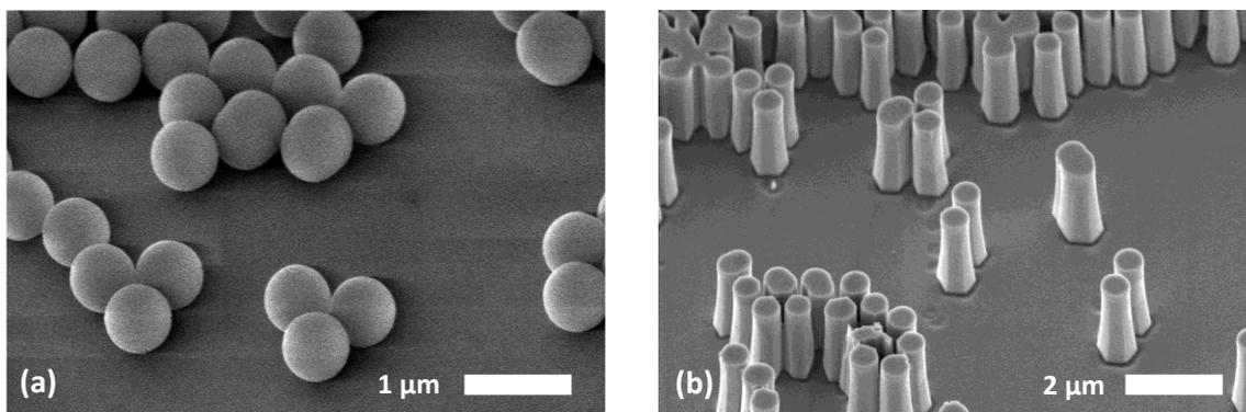
Figure 3.3.1: 700 nm SiO<sub>2</sub> nanospheres on a GaN surface (a). 3 μm tall GaN nanowires formed using 700 nm SiO<sub>2</sub> nanospheres as a dry etch mask (b).
