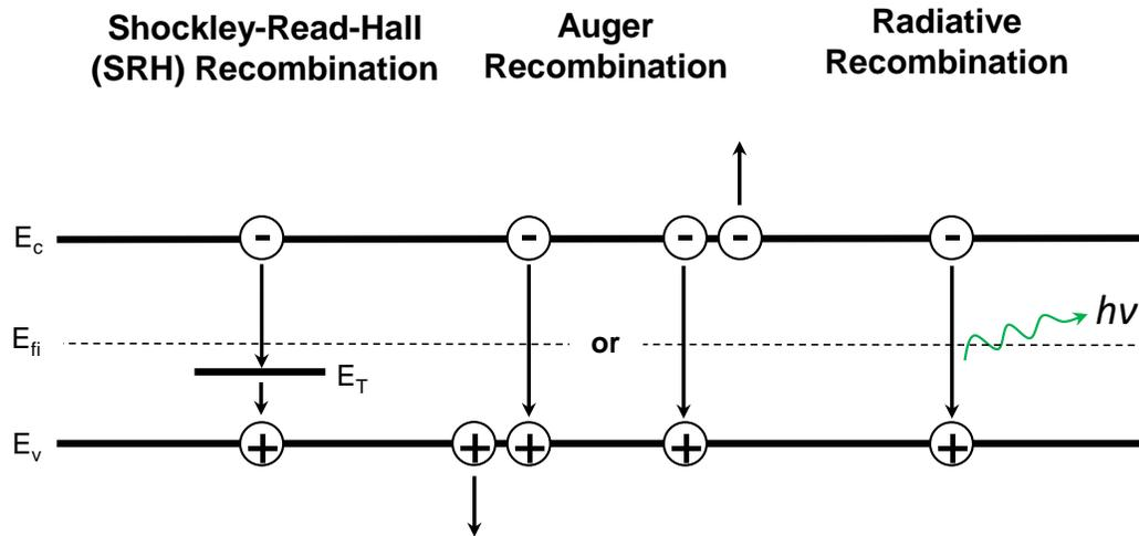
Figure 1.1.4: The three primary electron-hole recombination mechanisms likely to occur within the quantum wells of LEDs.
