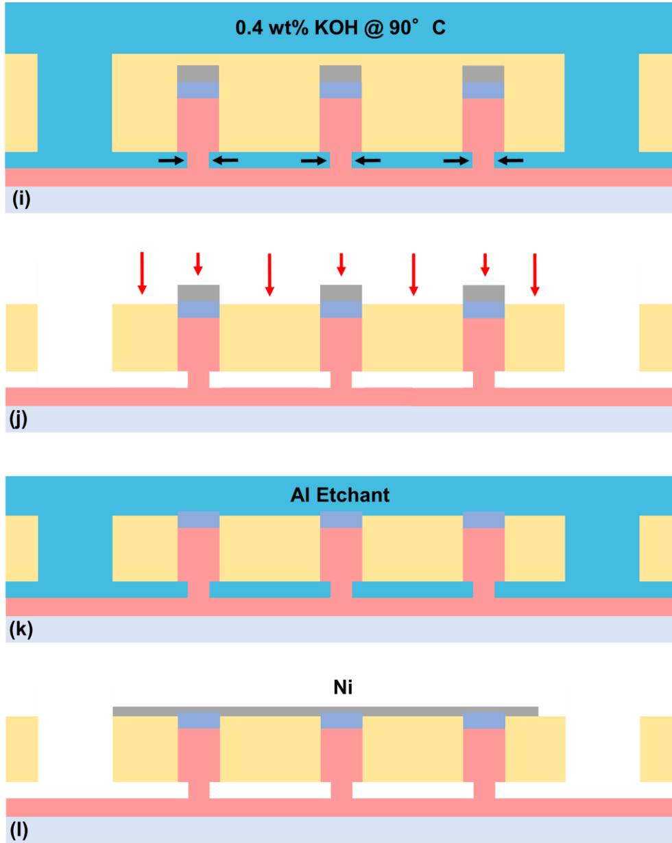
Figure 4.6.1(i-l): Narrowing or separation of the nanowire bases by a heated or room temperature KOH etch (i), etchback of the planarized  $\text{SiO}_2$  to expose the Al atop the nanowires (j), removal of the Al with a wet etch (k), deposition of a conformal connecting metal layer (Ni) onto the tops of the nanowires (l).
