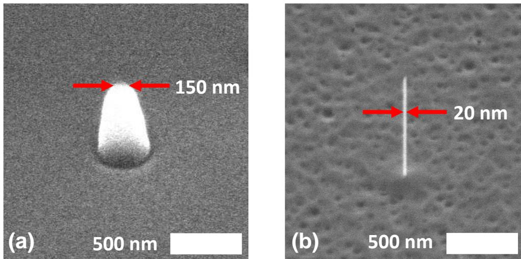
Figure 5.4.2: SEM images showing a nanowire after dry etch (a) and after 70 min in 40% AZ400K (b).
