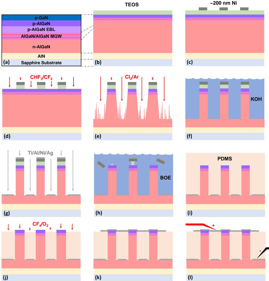
Figure 3.1.4: Nanowire LED fabrication schematic showing dry etch, wet etch, metallization, and dielectric planarization steps (not to scale).
