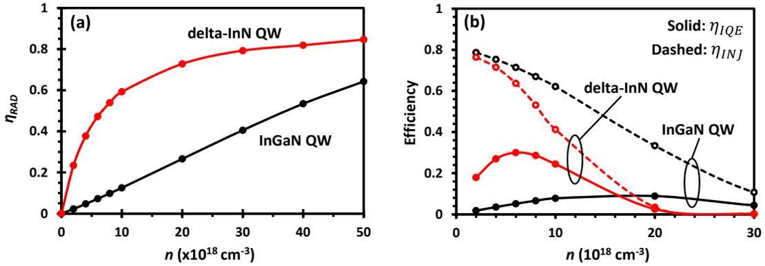
Figure 5.1.5: (a)  $\eta_{RAD}$ , and (b)  $\eta_{INJ}$  (dashed line) and  $\eta_{IQE}$  (solid line) for an  $\text{In}_{0.15}\text{Ga}_{0.85}\text{N}/\text{In}_{0.38}\text{Ga}_{0.62}\text{N}$  QW (black) and an  $\text{In}_{0.15}\text{Ga}_{0.85}\text{N}/\text{In}_{0.3}\text{Ga}_{0.7}\text{N}/\text{delta-InN}$  QW with a 3 Å delta-layer QW (red) as  $n$ . Both structures have  $\lambda_{\text{peak}} \sim 630 \text{ nm}$  at  $n = 5 \times 10^{18} \text{ cm}^{-3}$ .
