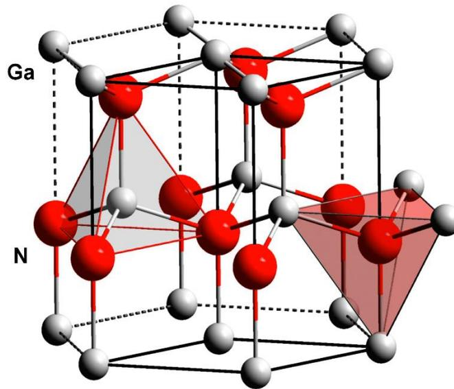
Figure 1.4.2: The wurtzite unit cell of GaN showing Ga atoms in white and N atoms in red [23].
