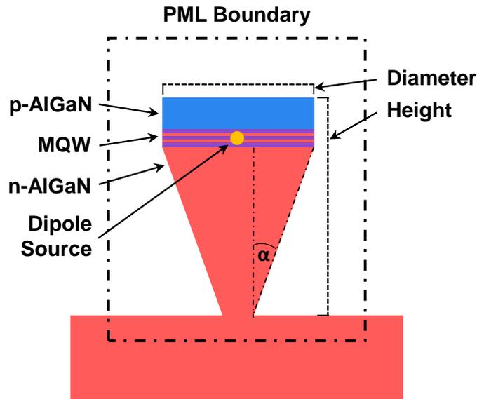
Figure 4.3.2: Cross sectional schematic showing a generalized representation of a simulated nanowire.
