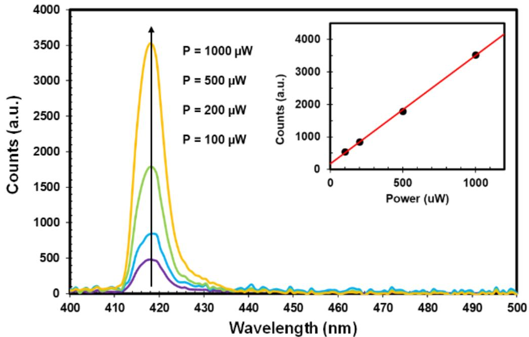
Figure 5.4.3: Power dependent PL spectrum of a single nanowire QD. Inset shows the linear dependence of emission intensity on pump laser power.
