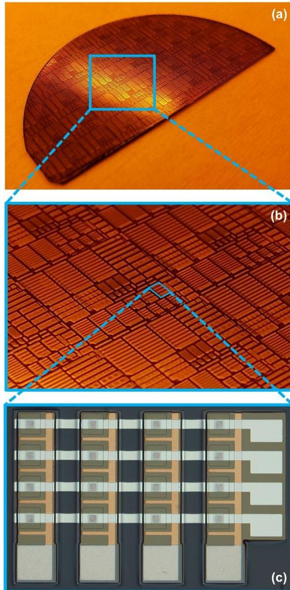
Figure 5.3.3: Images showing the passive matrix display samples at the wafer level (a), the die level (b), and the device level (c). The shown device is a 4x4 display with a pixel size of  $60\ \mu\text{m}$  and x/y pixel pitches of  $180/90\ \mu\text{m}$ .
