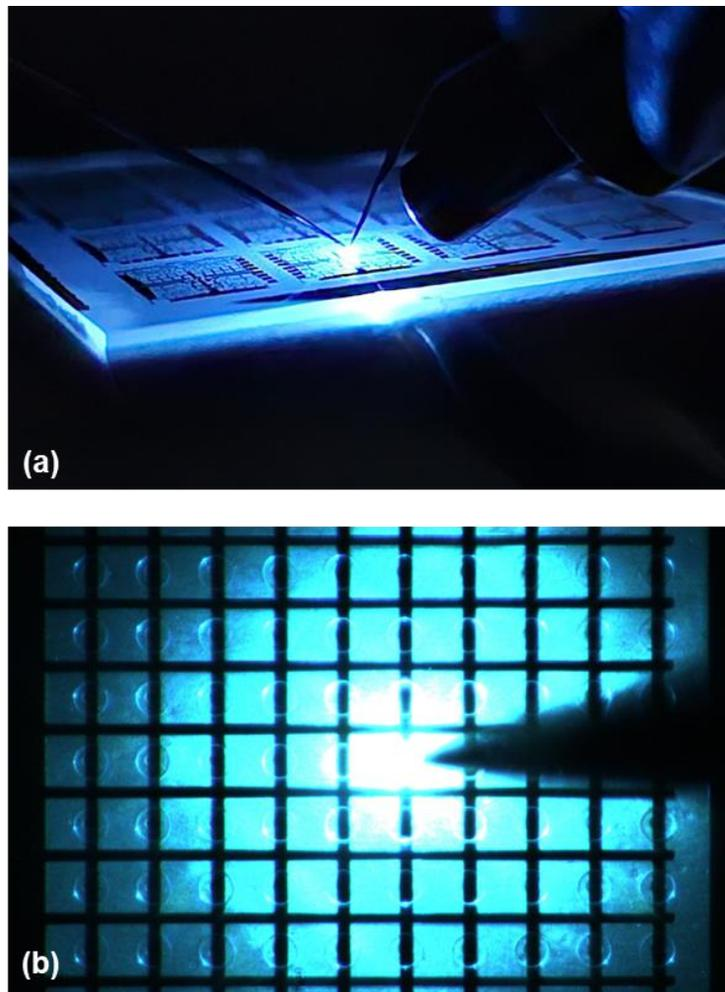
Figure 4.4.6: Illuminated 10 μm μLEDs imaged using a cell phone camera (a) and microscope camera (b). Despite narrowband emission occurring around 260 nm, cameras represent this emission as blue.
