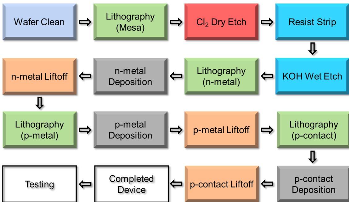
Figure 3.1.1: Mesa LED fabrication process flow with color coded process steps.
