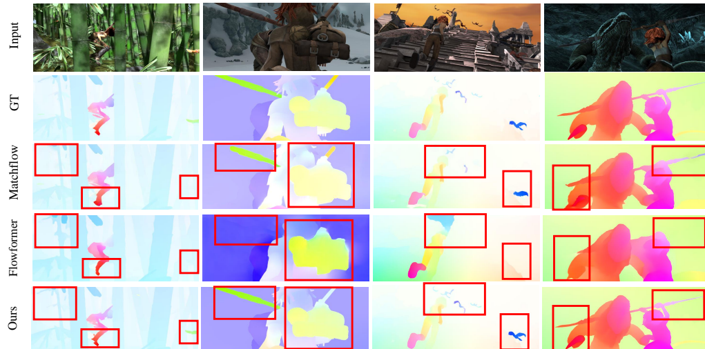
Figure 4.1: Qualitative results on the Sintel. The red boxes highlight the regions compared. Matchflow [28] appears blurry and ambiguous on textureless and occluded objects, while Flowformer [10] fails to recover complete and detailed information. Ours can estimate clear and complete flow motion, which is closer to ground truth.
