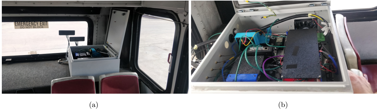
Figure 4.1: Example of POWDER mobile endpoint, deployed in University of Utah's campus shuttles: (a) – the location of the mobile endpoint inside the campus shuttle; (b) – a closer look to the employed hardware
