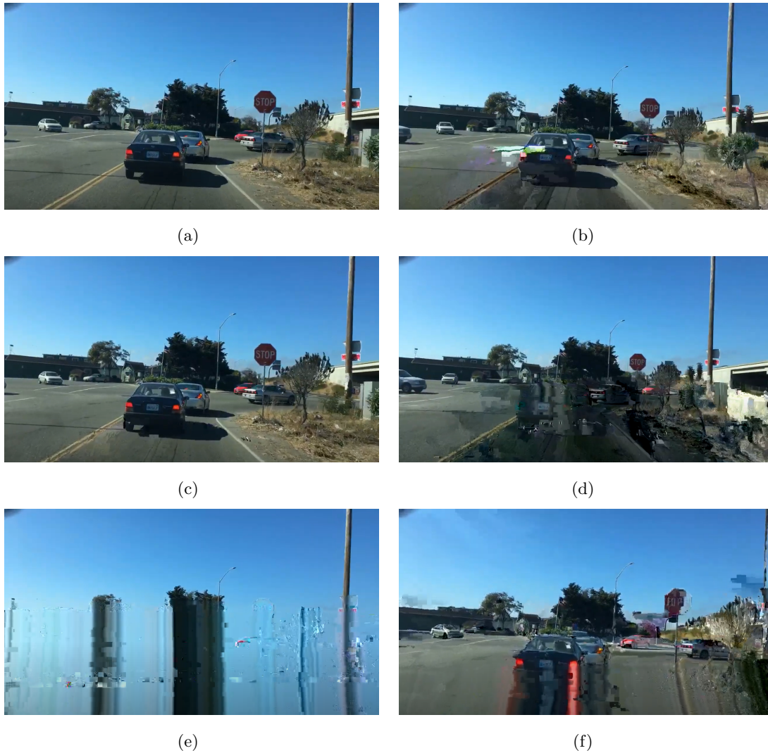
Figure 4.18: Examples of the frames from the road sign category video transmitted over a wireless network with 512B receiver buffer size and with packet loss rate of: (a) – 0%; (b) – 0.15%; (c) – 0.25%; (d) – 0.5%; (e) – 0.75%; (f) – 1%
