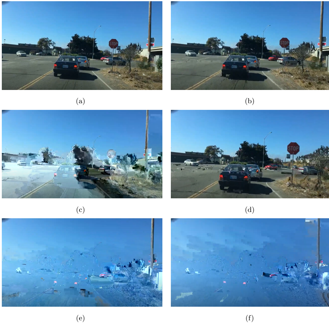
Figure 4.19: Examples of the frames from the road sign category video transmitted over a wireless network with 1024B receiver buffer size and with packet loss rate of: (a) – 0%; (b) – 0.15%; (c) – 0.25%; (d) – 0.5%; (e) – 0.75%; (f) – 1%
