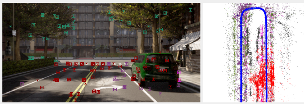
Figure 2.1: ORB feature extraction (left) and top down view of sparse 3D map (right)
