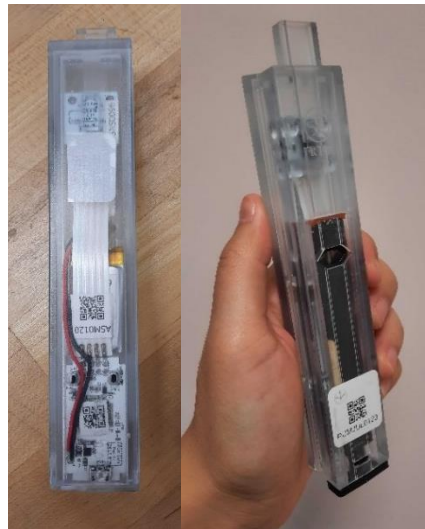
Figure 20. The JUUL monitor used Gen 3 (A+). The see-through material on the right side shows the internal electronics, while the left side shows the monitor held by a user.
