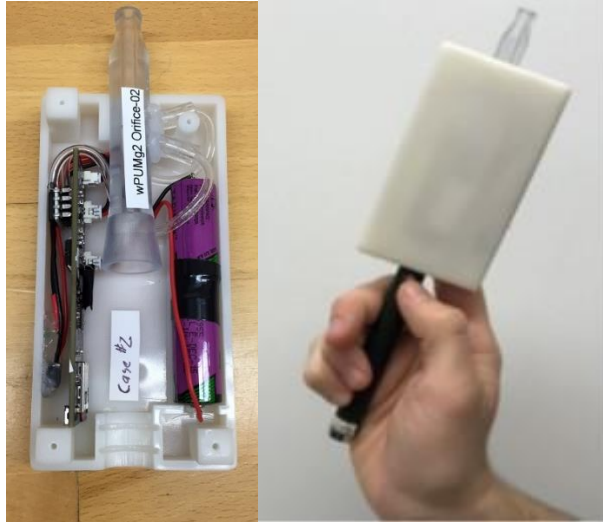
Figure 16. The pen-style monitor used Gen 2 long-version electronics.
