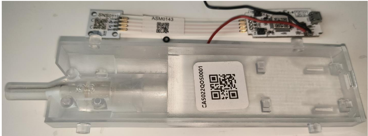
Figure 62. The disassembled monitor, the electronics assembly of 3 inches (top), and the electronics housing (bottom).
