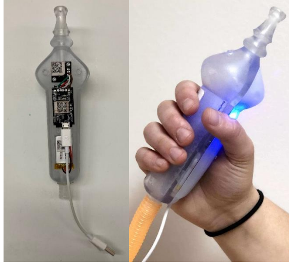
Figure 19 The Hookah monitor used Gen 3 (A) and (A+). The left side shows the internal electronics, while the right side shows the monitor connected to an actual hookah hose held by a user.
