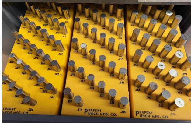
Figure 42. The gauge pin tray test is used to measure the inner diameter of the interface cone.
