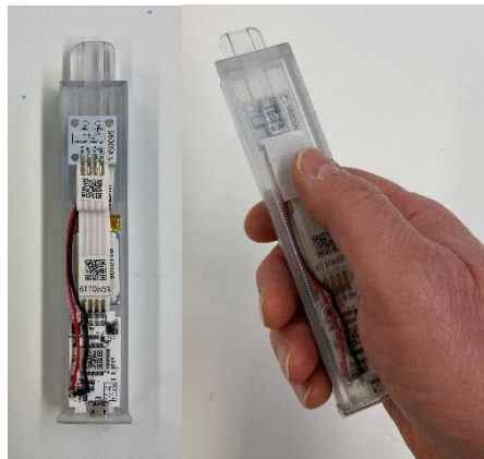
Figure 22. Hyde original monitor used Gen 3 (A+) electronics as seen on the left side and the monitor in use on the right side.
