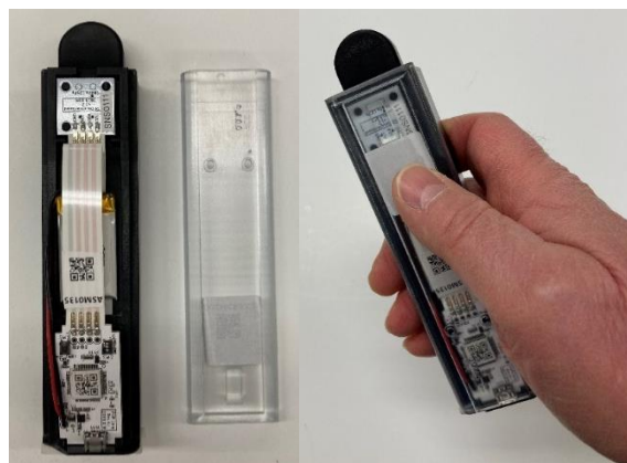
Figure 23. Ace monitor with the electronics Gen 3 (A+) inside and the handheld.
