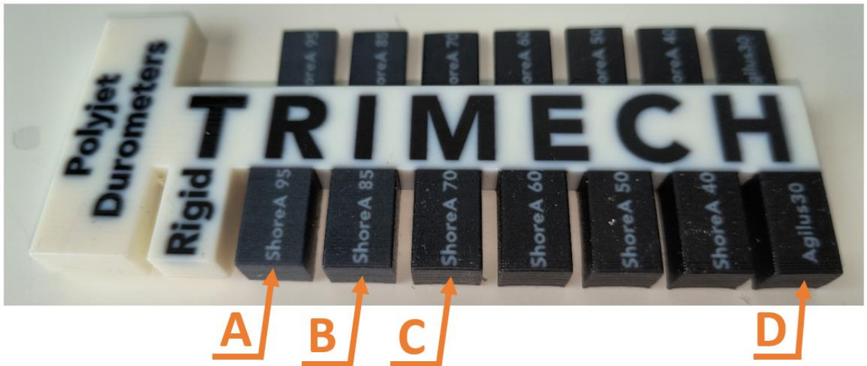
Figure 47. A sample piece has different Polyjet machine shore values that TriMech can afford.
