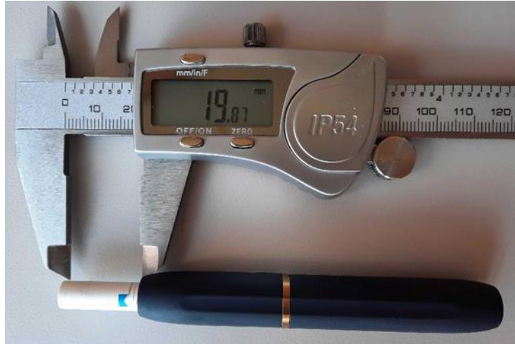
Figure 38. Exposed part of the heat stick after being inserted into IQOS
