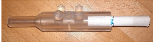
Figure 12. The initial design of the mouthpiece. This part was the core of our monitor, as it was validated and tested in a previous study.
