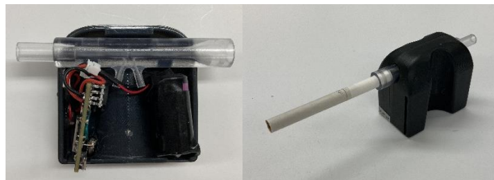
Figure 15. Gen 2 short-style electronics are used for cigarette monitors.
