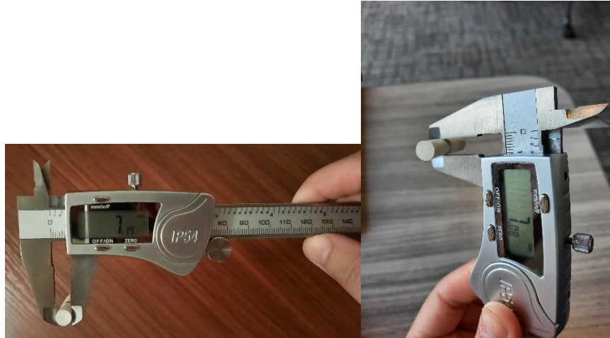
Figure 35. Using the caliper to measure the diameter of the heat stick, (left) is displayed at 3mm from the tip, and (right) is at 20 mm from the tip.
