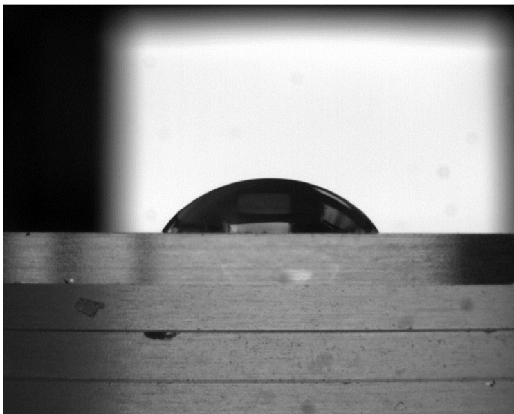
Figure 13 - Glass sample treated with a 10% n-Decyltrichlorosilane, 97% solution in ethanol. The contact angle between the droplet of water and the glass slide is measured at 49^\circ
