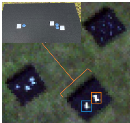
Fig. 2. Zoom of Fig. 1 showing deployment of mirrors. Upper left shows photo of physical mirror layout. Box colors align with the reflectance curves in Fig. 3.
