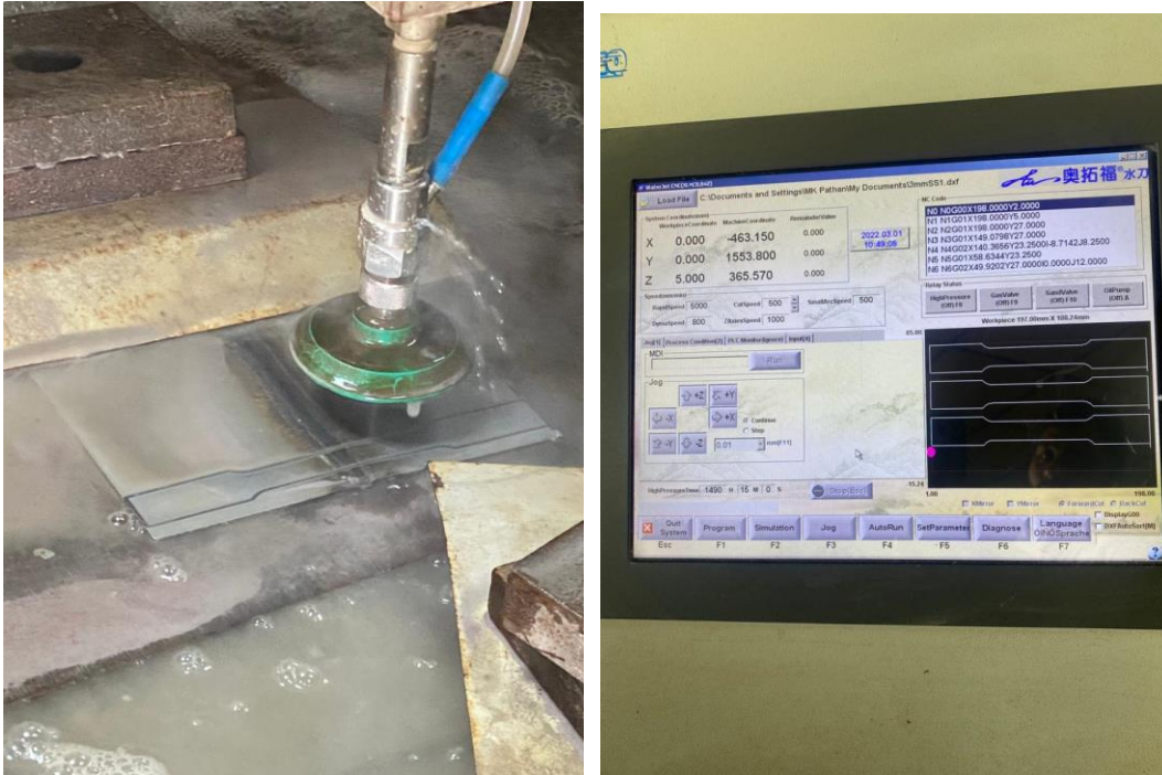
Figure 2. Preparation of tensile test specimen using water jet machining
