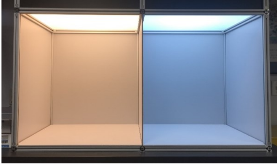
Figure 4.1: Bipartite light booth used in chromatic adaptation experiments.
