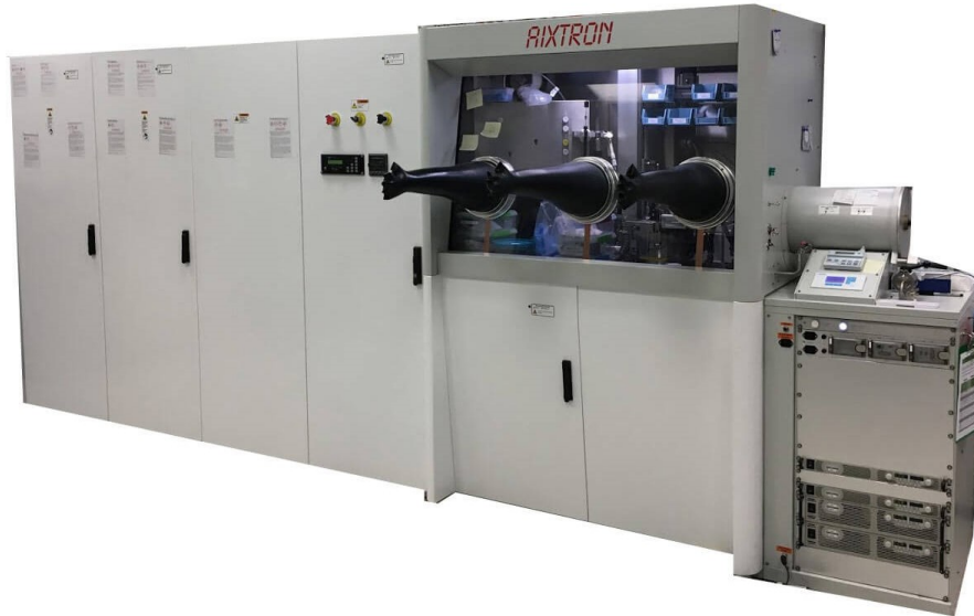
Figure 2.2. Aixtron 3×2" CCS MOCVD reactor operated within the NanoPower Research Laboratories (NPRL) at RIT.
