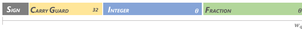
Figure 2.13: Illustration of Quire format with variable IS and SC (e.g, the quire size for 8-bit tapered fixed-point with IS = 8 and SC = 0 is 50 bits)
