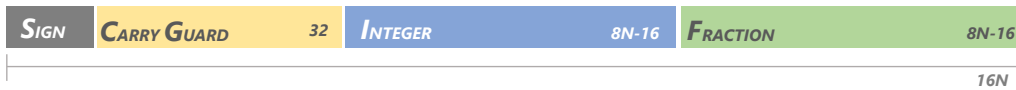
Figure 2.5: Illustration of quire format with 2-bit exponent ( e_s = 2 ). For instance, the quire size for 8-bit posit with e_s = 2 is 128 bits).
