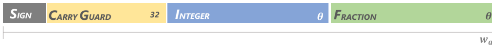
Figure 2.9: Illustration of quire format with variable es and rs (e.g, the quire size for 8-bit posit with es = 2 and rs = 3 is 80 bits)
