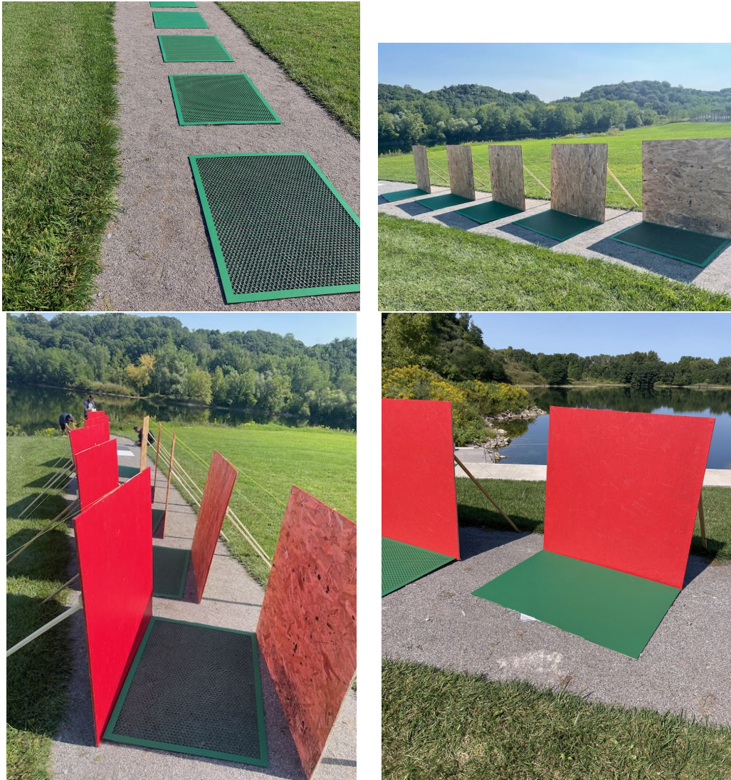
Figure 3.3: The four target setups used at Tait Preserve for the data collect. The top-left image shows the base setup of green sub-pixel targets with no shadowing or TR panels. The 20% FF target is closest in the field-of-view (FOV). The top-right image shows the shadowing panel setup. The bottom-left image shows the TR panel and shadowing panel (TR-S) setup. The TR panel setup is shown in the bottom-right image. The spectral contamination from the TR panel may be seen on the shadowing panel in the bottom-left image.
