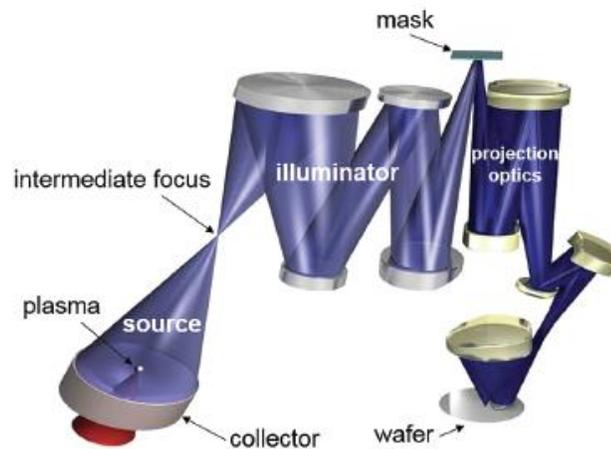
**Figure 1.7: Schematic of a typical 0.33NA EUVL system from ASML.**
