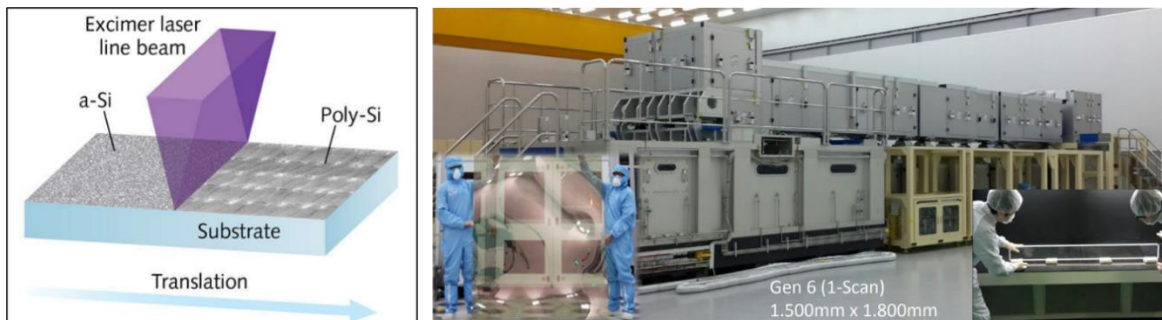
Figure 1.4: Diagram of ELA scanning process and photograph of a modern ELA system capable of crystallizing Gen 6 glass in a single scan. Adapted from [14]
