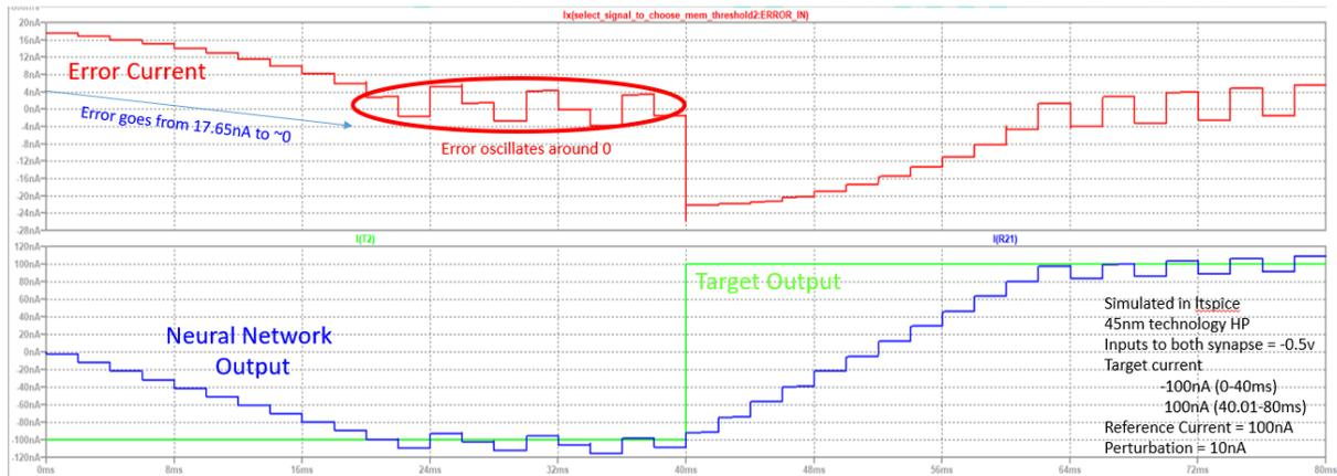
**Figure 7.5:** The simulation waveform of the Error Calculation
