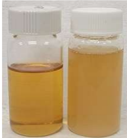
Figure 2 Clean 10W30(left) and contaminated 10W30 (Right)
