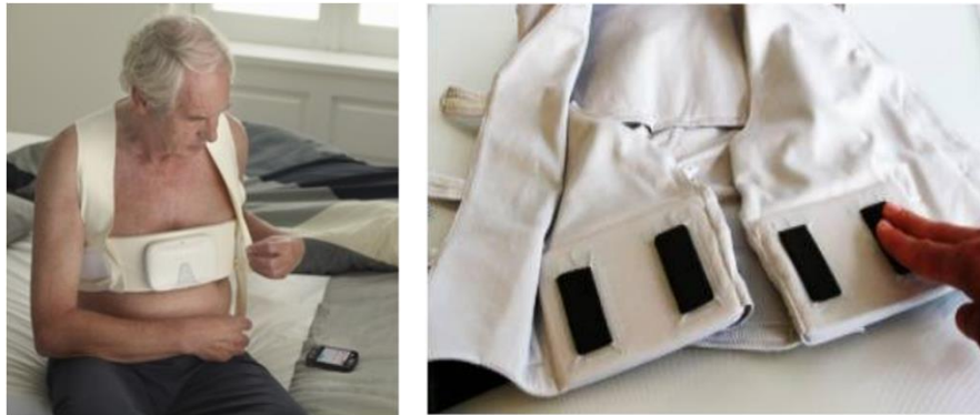
Figure 1.4: Wearable vest for measuring transthoracic impedance with four embedded textile-based electrodes [16], [17].
