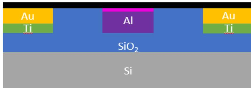
Fig. 52:- Schematic of a dual back gated fabricated at RIT SMFL with source/drain metal contacts (Au/Ti) (95/5)nm with 200 nm of aluminum and 300 nm of  $SiO_2$ .
