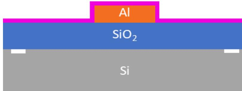
Fig. 46 :- A bare P-Type Si wafer (grey) with 90 nm of dry oxide growth of  $SiO_2$  on it (blue), with the aluminum gate (orange), TEOS deposition is done on top of aluminum gate (pink).
