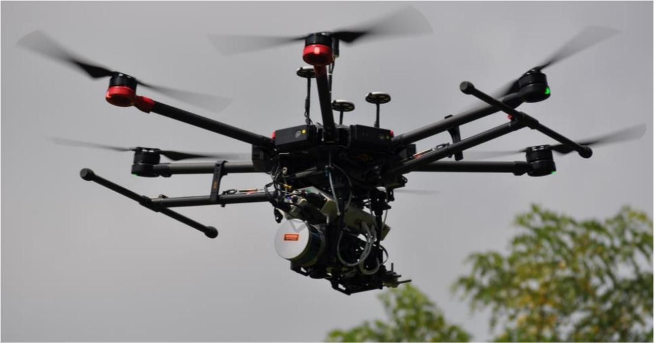
*Figure 7: The first set of simulated data is based on truth data from the Velodyne VLP-16 lidar sensor, which is integrated on a Matrice 600 unmanned aerial system (UAS). The drone is a MX-1 sUAS remote sensing platform, developed by CIS faculty at RIT. Additionally, the drone contains a Mako G-419 RGB camera and ballast weight in place of the hyper-spectral camera [40].*
