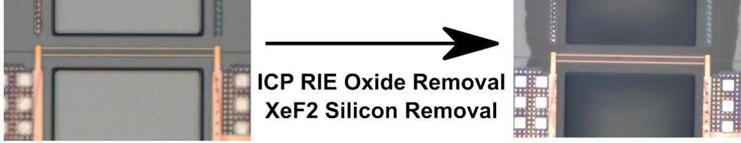
Figure 4.3: A before and after microscope image of the ICP RIE oxide removal and XeF<sub>2</sub> silicon removal etches, we see on the right-hand side that the silicon handle is removed below the device,
