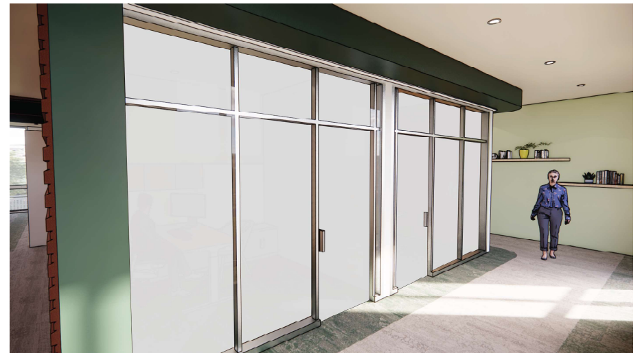
Fig. 57: Private Offices - Switch-Glass On
