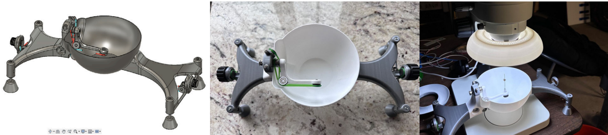
Figure 14: This prototype shows the first integration of integrating sphere, positioned arm, and upper light.
