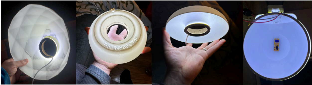
Figure 13: These lighting prototypes used a variety of LED ring lights and the two center images show the most successful design that attaches to the microscope and provides the most diffuse light.
