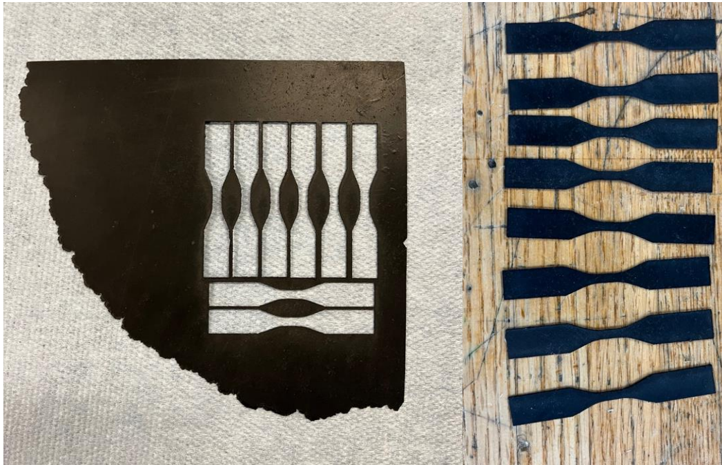
Figure 3: Dog bone created by laser cutting after composite pressing
