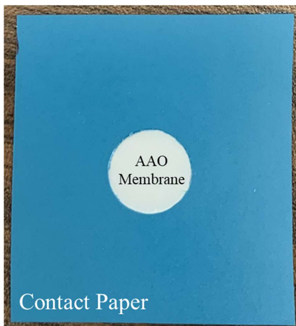
Figure 2: AAO membrane embedded in two pieces of contact paper. Both pieces of contact paper have a 13mm hole that is lined up with the 15mm AAO membrane.
