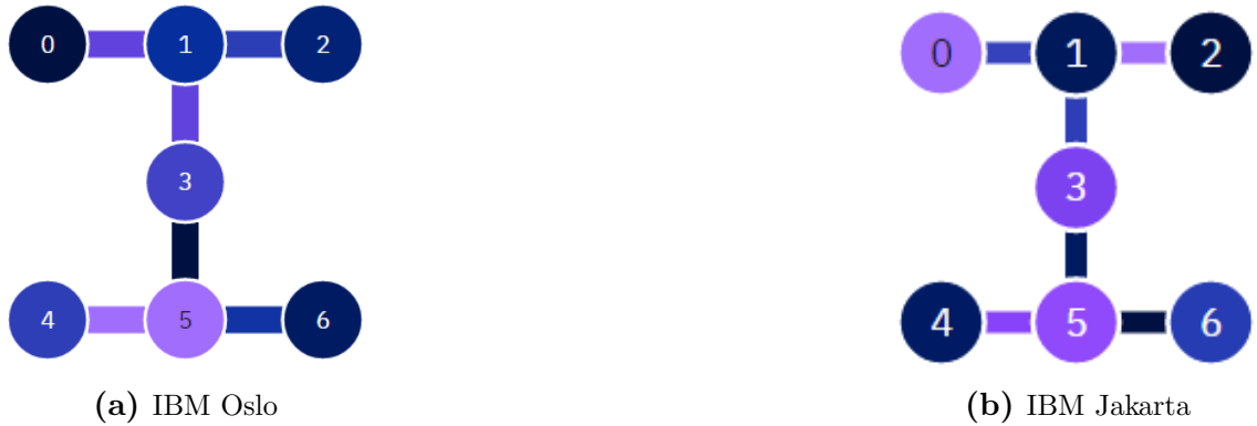
Figure 2.4: Different errors for different 7-Qubit IBM Falcon r5.11H Quantum Processors. Link colors correspond to CNOT link error, where lighter links have a higher error rate than darker links.
