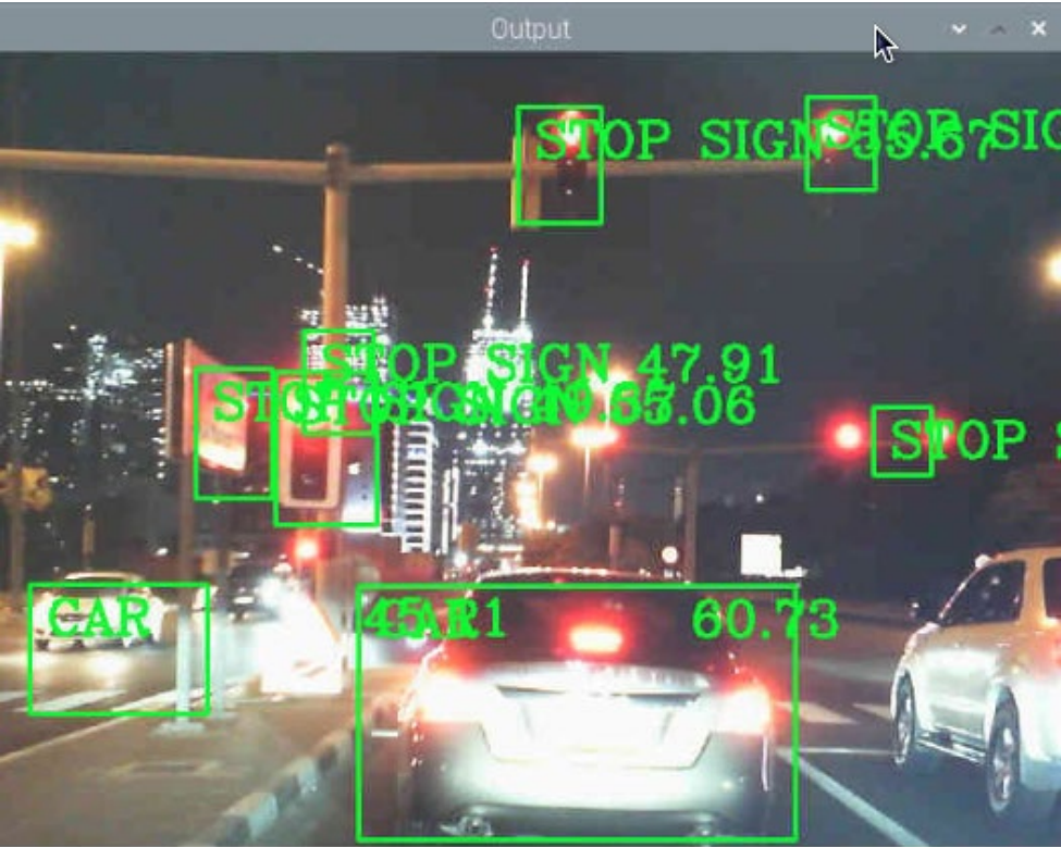
Figure 29 Example of Street Objects Detected using the Camera Module
