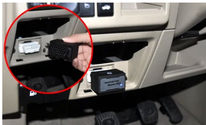
Figure 20 OBDII Scanner and Location in Vehicles
