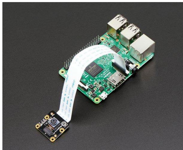
Figure 19 PiCamera Module Connected to Raspberry Pi
