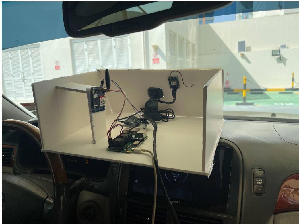
Figure 39 Vehicle Agent Installation Inside a Vehicle
