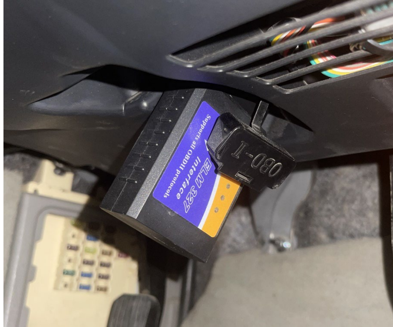
Figure 34 OBDII Scanner Connection
