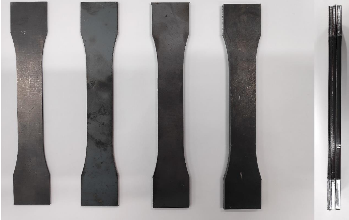
Figure 13 - Unpainted coupons of 1-4 mm
