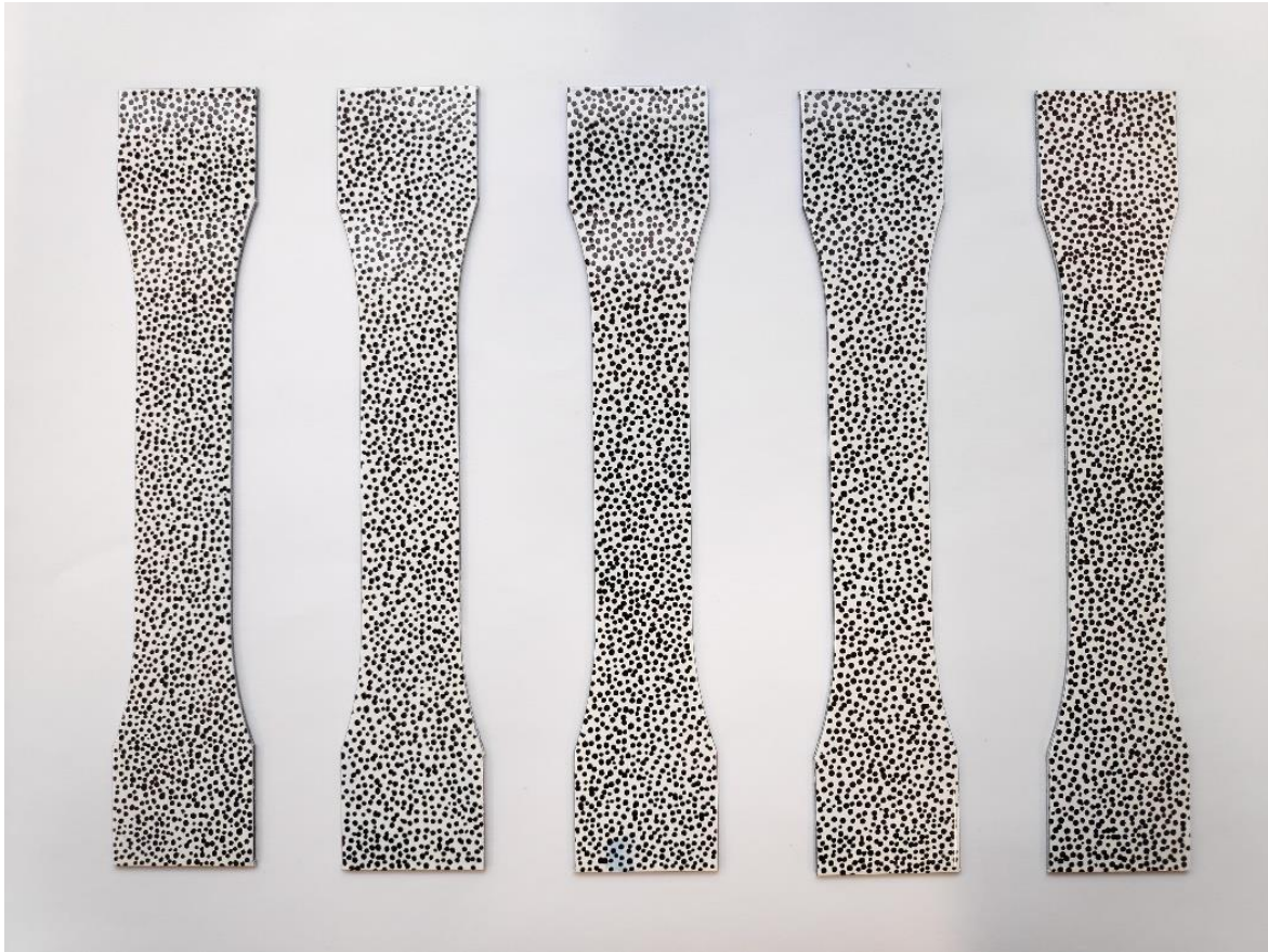
Figure 16 - Specimens with paint and speckle pattern applied
